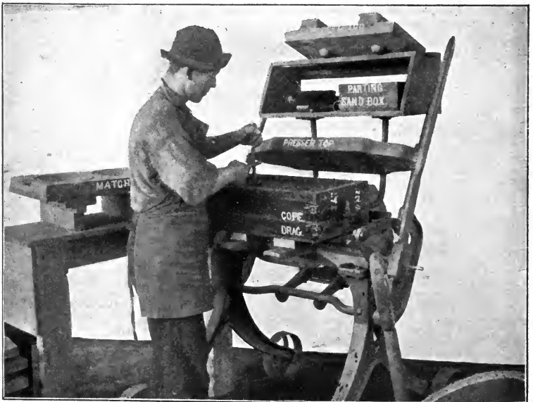
FIG. 207. — RAPPING THE PATTERN BEFORE SEPARATING THE MOLD.
