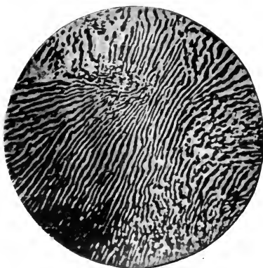
FIG. 241. — PEARLITE EUTECTOID OF IRON AND CARBON. (F. Osmond.)
