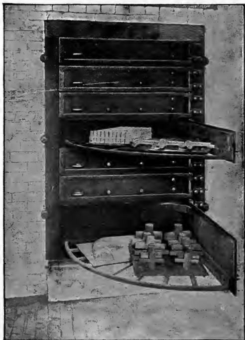
FIG. 201. — OVEN FOR DRYING SMALL CORES.
