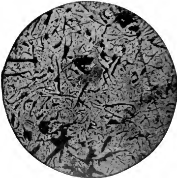
FIG. 260. — GRAY PIG IRON. 1.75 per cent. Si. 0.025 per cent. S. S. 50 diameters. Unetched.
