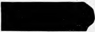
FIG. 132.—SHAPE OF ENDS OF ROLLED METAL WHEN THE INSIDE IS THE HOTTER.
