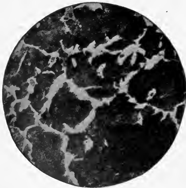
FIG. 291. — FERRITE AND SORBITE IN RAILED STEEL.
