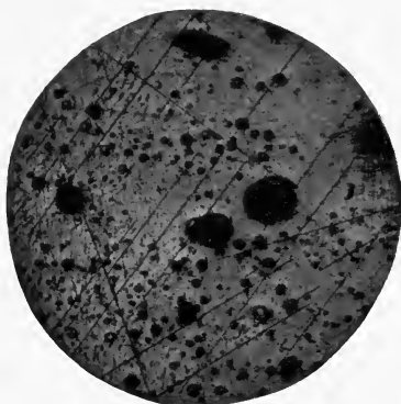
STRAIGHT SLIP BANDS IN WROUGHT IRON MAGNIFIED 60 DIAMETERS.
