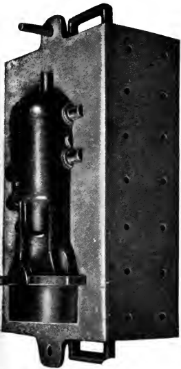
FIG. 188. — MAKING THE MOLD. Pattern in the sand of lower section of flask.
