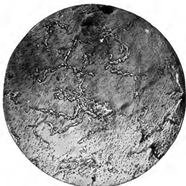
FIG. 297. — 0.41 PER CENT. CARBON. COOLED EXTREMELY SLOWLY. Magnified 265 diameters. Etched with picric acid.
