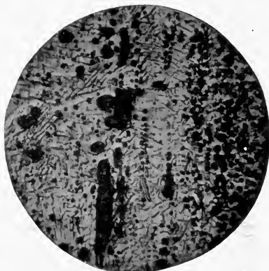
CURVED SLIP BANDS IN WROUGHT IRON MAGNIFIED 60 DIAMETERS.
