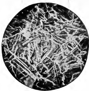
FIG. 292. — 1.54 PER CENT. CARBON. ROLLED. Magnified 225 diameters. Etched with picric acid.
