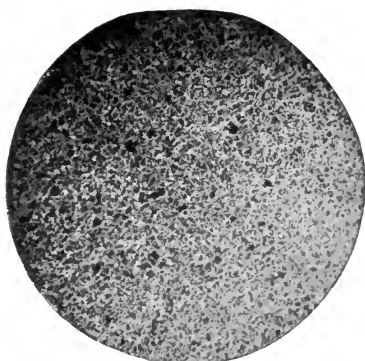
FIG. 278. — NO. 1B. STEEL OF 0.50 PER CENT. CARBON ROLLED. Magnified 60 diameters.
