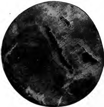
FIG. 252. — ELONGATED BUBBLE OF MANGANESE SULPHIDE. Magnified 250 diameters. Unetched.
