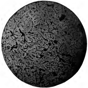
FIG. 259. — GRAY PIG IRON. 0.75 per cent. Si. 0.012 per cent. S. S. 50 diameters. Unetched.
