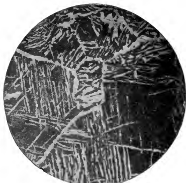
FIG. 280. — NO. 2B. SAME AS NO. 1B. OVERHEATED TO 1420° C. (2588° F.) Magnified 60 diameters.
