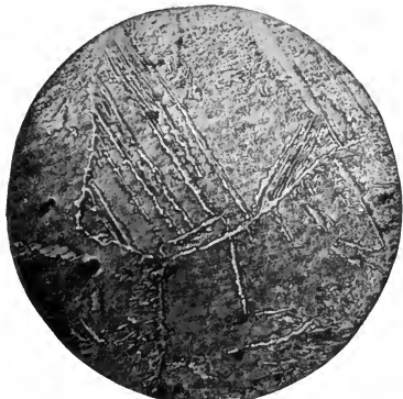
FIG. 295. — 1.24 PER CENT. CARBON. COOLED EXTREMELY SLOWLY. Magnified 265 diameters. Etched with picric acid.
