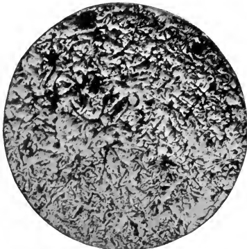
FIG. 262. — GRAY PIG IRON. 3.5 per cent. Si. 0.025 per cent. S. S. 50 diameters. Unetched.
