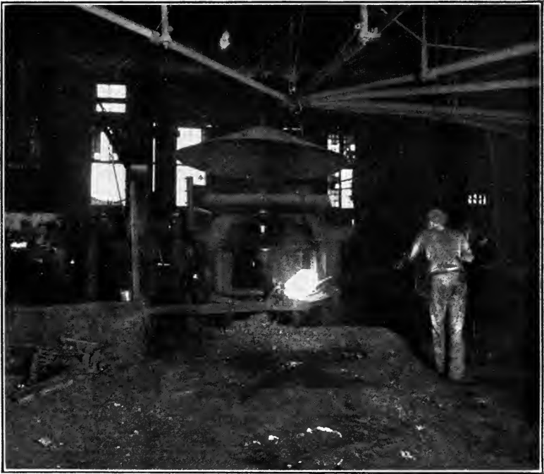
FIG. 49.—THE BALL ENTERING THE SQUEEZER.
