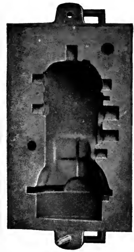
FIG. 189. — MAKING THE MOLD. Pattern removed from sand showing molded impression.
