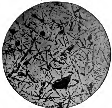
FIG. 261. — GRAY PIG IRON. 2.5 per cent. Si. 0.012 per cent. S. S. 50 diameters. Unetched.
