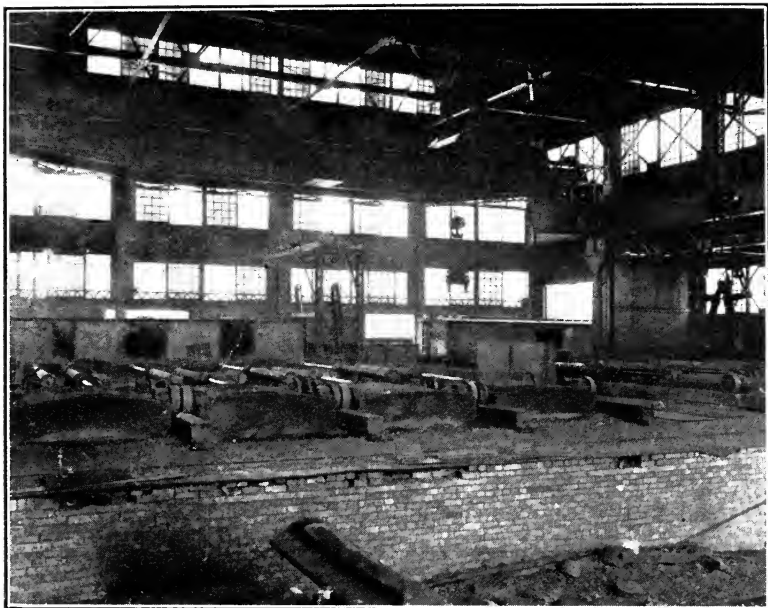
FIG. 80. — SOAKING PIT HEATING FURNACES AT ROLLING MILL WHICH RECEIVE THE RED HOT, NEWLY STRIPPED INGOT.
