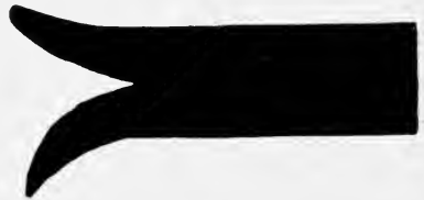
FIG. 133.—SHAPE OF ENDS OF ROLLED METAL WHEN THE OUTSIDE IS THE HOTTER.
