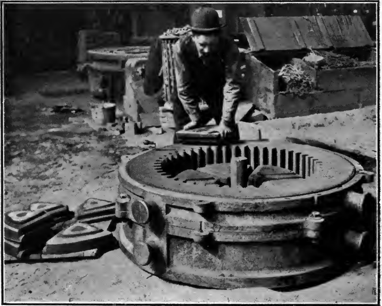
FIG. 187. — PLACING CORES IN A MOLD.
