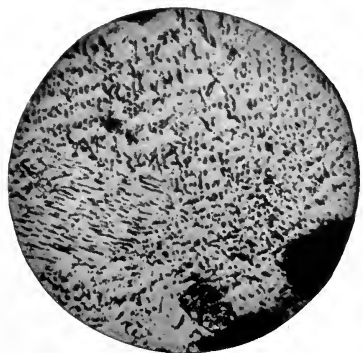
FIG. 253. — EUTECTIC OF \text{Fe}_3\text{P} AND IRON. Magnified 1000 diameters. Etched with picric acid.
