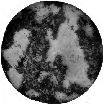
FIG. 289. — MARTENSITE (WHITE) AND TROOSTITE (DARK).
