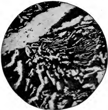
FIG. 250. — BIG CEMENTITE CRYSTAL IN PEARLITE. Magnified 250 diameters. Polished in relief.
