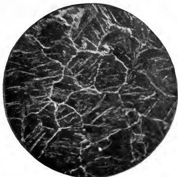
FIG. 293. — 1.24 PER CENT. CARBON. ROLLED. Magnified 225 diameters. Etched with picric acid.
