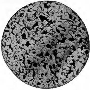
FIG. 286. — NO. 2A. SAME AS NO. 1A. REHEATED SLIGHTLY ABOVE AC_3 .
