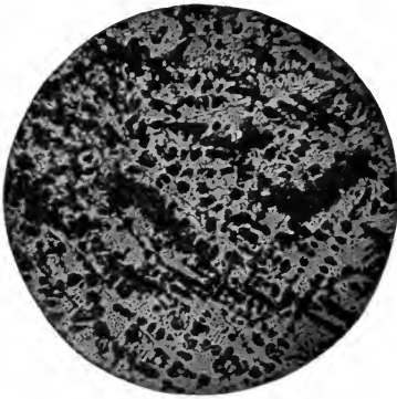
FIG. 258. — WHITE PIG IRON. 0.75 per cent. Si. 0.120 per cent. S. 50 diameters. Unetched.
