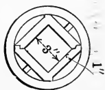
FIG. 60. — INGOT MOLD FOR CRUCIBLE STEEL. From Howe, "The Metallurgy of Steel."
