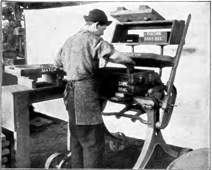
FIG. 206. — CUTTING SPRUE WITH TUBULAR SPRUE CUTTER.
