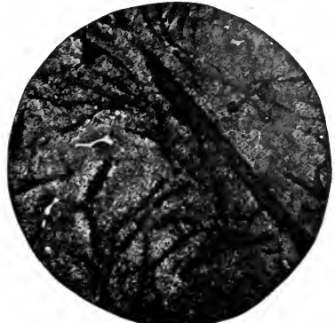
FIG. 263. — NO. 2 CHARCOAL PIG IRON VERY SLOWLY COOLED. 50 diameters. \text{HNO}_3 .
