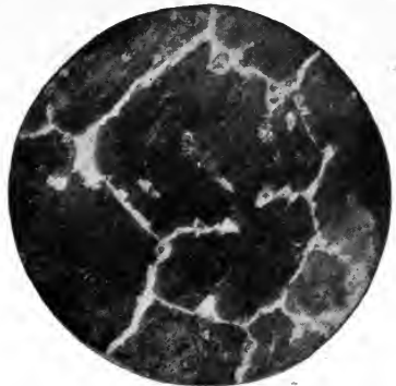
FIG. 249. — PEARLITE CRYSTALS. Surrounded by ferrite. Magnified 250 diameters. Etched with \text{HNO}_3 .
