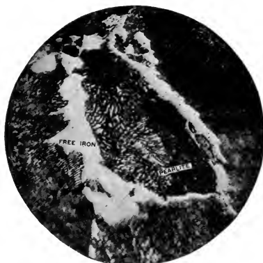
FIG. 242. — PEARLITE AND FERRITE. 250 diameters.
