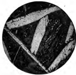
FIG. 251. — CRYSTALS OF MANGA- NIFEROUS CEMENTITE. Magnified 50 diameters. Etched with nitric acid.
