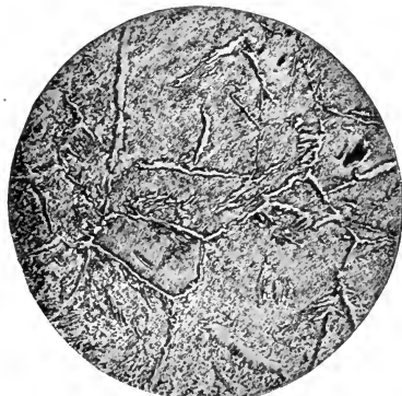
FIG. 296. — 1.24 PER CENT. CARBON. COOLED EXTREMELY SLOWLY. Magnified 265 diameters. Etched with picric acid.
