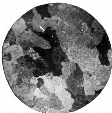
FIG. 279. — NO. 2A. SAME AS NO. 1A OVERHEATED TO 1420° C. (2588° F.) Magnified 40 diameters.
