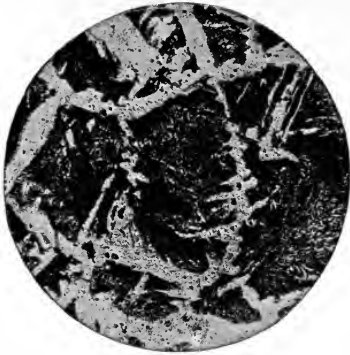
FIG. 285. — NO. 1A. STEEL OF 0.34 PER CENT. CARBON OVERHEATED TO ABOUT 1300° C. (2372° F.).
