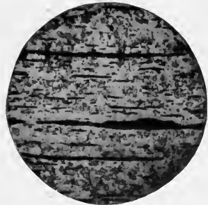
FIG. 52. — WROUGHT IRON SHOWING STRINGS OF SLAG MAGNIFIED 50 DIAMETERS.
