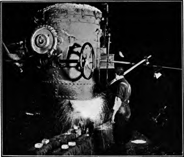
FIG. 77. — TEEMING INTO MOLDS.
