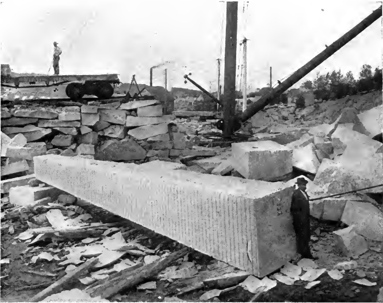
FIG. 14.—A Spire of Barre (Vt.) Granite Over 60 Feet Long, Showing Marks of Drills, Also Showing Shallow Holes on End for Plug and Feathers.
