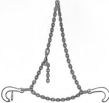
FIG. 71.—Forged Steel Grab Hooks and Chain. X Varies from 7 to 10 Inches. Capacity Varies from 2\frac{1}{2} to 25 Tons. (American Hoist and Derrick Co.)
