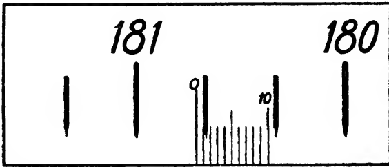
FIG. 17—Estimating microscope, direct reading = 180^{\circ} \cdot 43'
