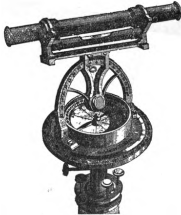
Simple English Theodolite of last Century, now commonly known as Lean's Dial.
