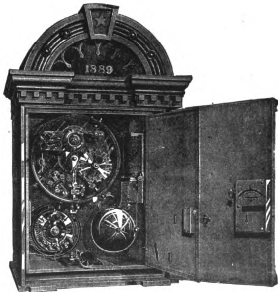
GAYNOR FIRE ALARM STREET BOX.
