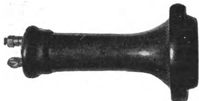
FIG. 32.— ASSEMBLED BELL RECEIVER (COMMON BATTERY TYPE).
