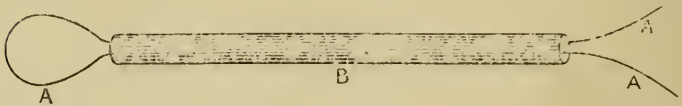
Snare for Extracting Puppies, Made Out of Flexible Copper Wire (A) and a Nickel-plated Thermometer Case (B). A Safe and Efficient Substitute for the Ordinary Forceps. Especially Useful in Small Bitches.
