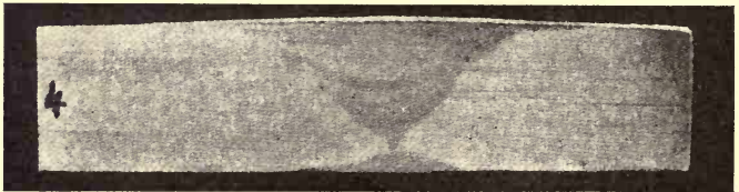
FIG. 55.— Traces of carbon deposits in a welding seam.
