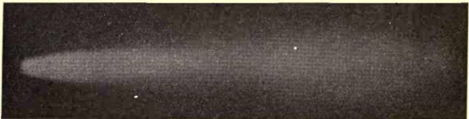
FIG. 39. — Carbonizing welding flame, i.e. with excess of acetylene.
