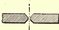
FIG. 69.—Double bevelling of edges of very thick sheets ( \frac{1}{2} inch or over) for welding purposes.
