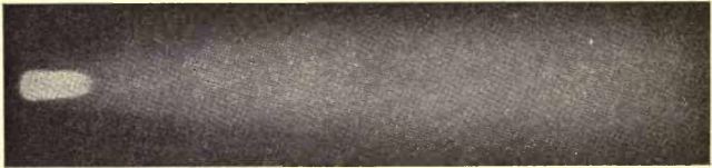
FIG. 38. — Correctly adjusted or neutral oxy-acetylene welding flame.
