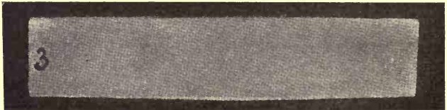
FIG. 52. — Etching of a good welding seam.
