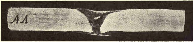
FIG. 56.— Excessive carbonization in a welding seam.
