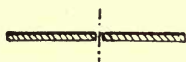
FIG. 67.—Butting together the edges of sheets for welding purposes. This method is satisfactory for sheets up to \frac{3}{32} inch in thickness.
