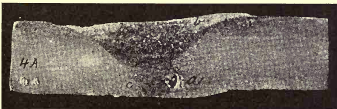
FIG. 73.— Superheated and carbonized welding seam containing foreign matter (a. b. c.).
