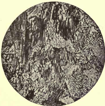
FIG. 46. — Micro-photograph of steel bar containing about 0.75% carbon. (Magnified 300 diameters)
