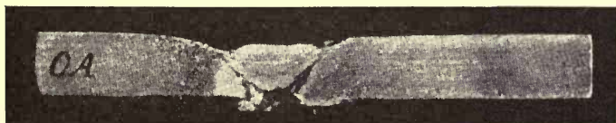
FIG. 77.— Example of bad welding.
