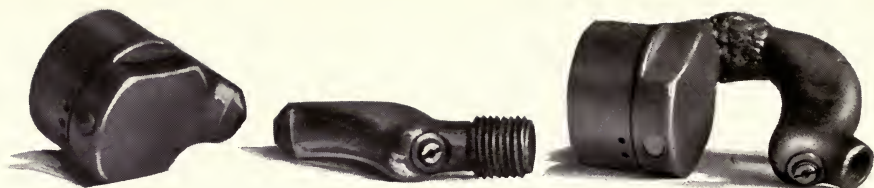
No. 1 Reclamation of Pneumatic Hammer Handle
