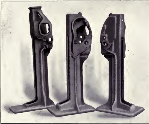
Samples of Welded Cast Iron and Steel, Wrought Iron and Boiler Plate
