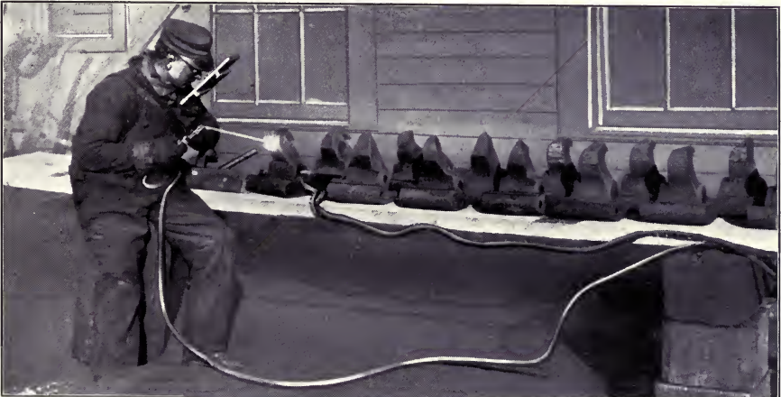
Reclamation of Freight Car Knuckles on a Trunk Line. The saving in one year on this item alone was more than $20,000.00.
