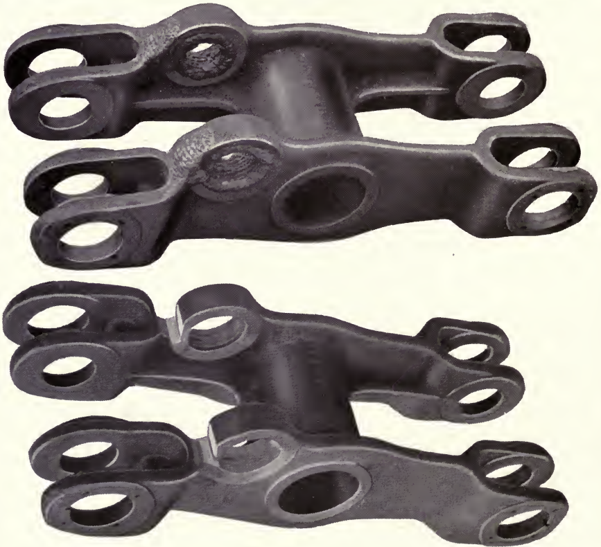
Damaged Walking Beam Circulating Pump, U. S. S. Drayton Cost $2.35 Saving $17.50
