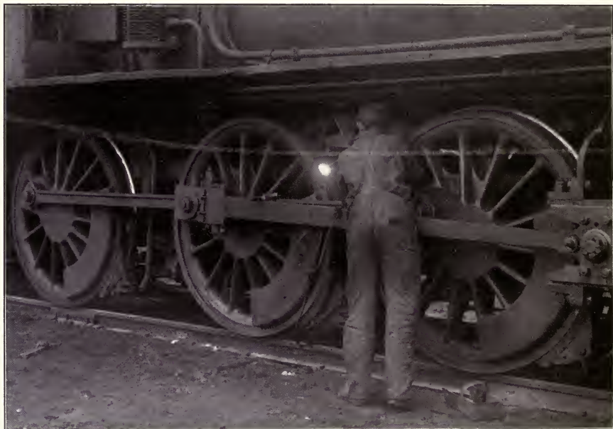
Building up Flat Spots on Locomotive Drivers.
