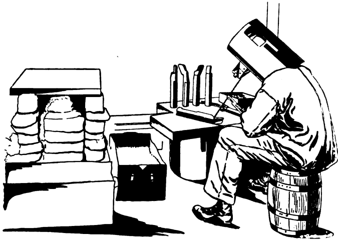
FIG. 147.—Welding High-Speed Tips Onto Mild Steel Shanks.
