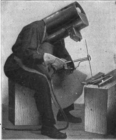
Fig. 36.—Correct Welding Posture and Equipment.
