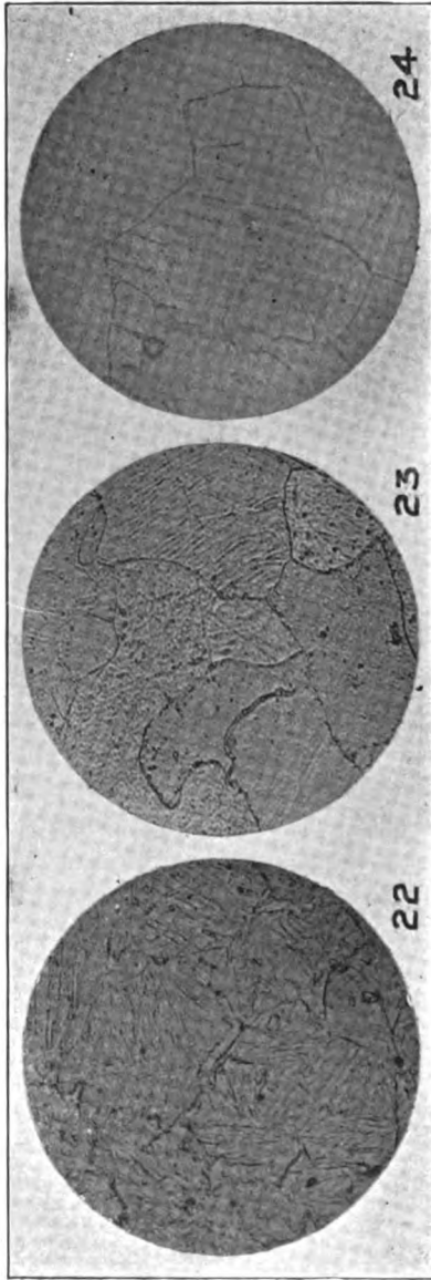
FIG. 164.—(22) Specimen AD 2 Quenched in Cold Water from 1000 Deg. C., Suppressing Nitride Plates and Developing Martensitic Structure. Etched with 5 Per Cent Alcoholic Picric Acid. \times 500 .
