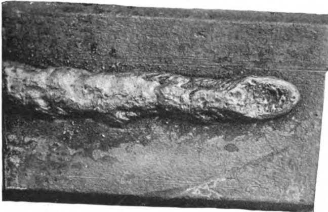
FIG. 52.—Method of Depositing Filling Material in Layers.
