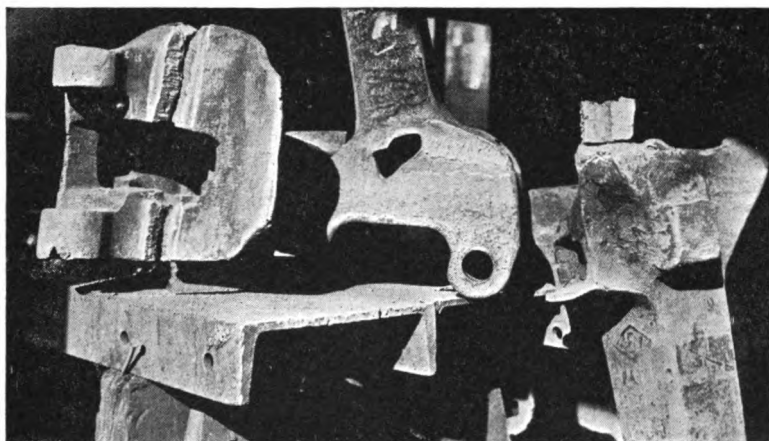
FIG. 28.—Car coupler used in railway work before arc welding.
