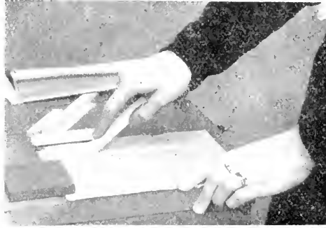
FIG. 46. ROUNDING ENDS ON GLASS PAPER.
