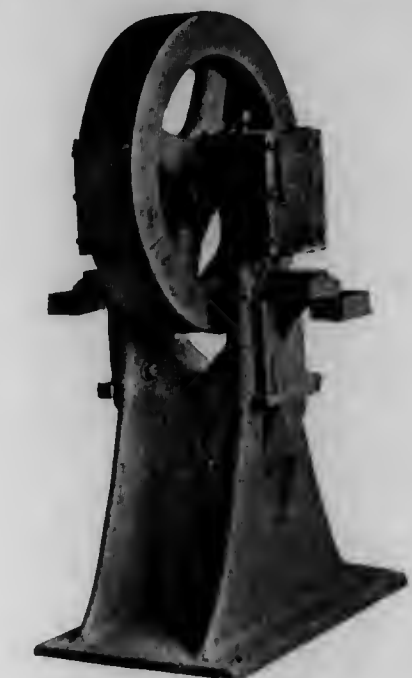
HEADING ROUNDER Now made with Ball Bearing Arbor
