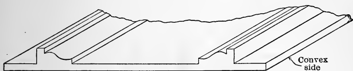
FIG. 7.—Thin Flat Plates, Unequal Shrinkage.
