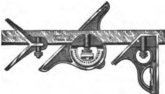
FIG. 25. COMBINATION SQUARE, MITER AND INCLINOMETER
