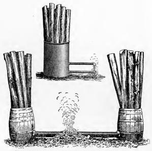
FIG. 77.—Simple apparatus for treating posts.<sup>1</sup>
