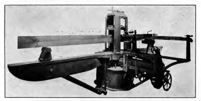
FIG. 32.—Machine for testing heavy wooden beams.<sup>1</sup>
