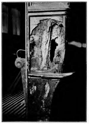
FIG. 79.—Failure of car post due to application of paint upon imperfectly seasoned wood.
