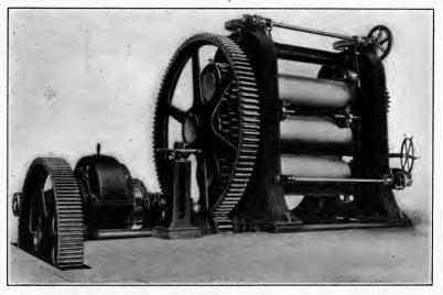
FIG. 90.—Calender with coil clutch motor drive.<sup>1</sup>
