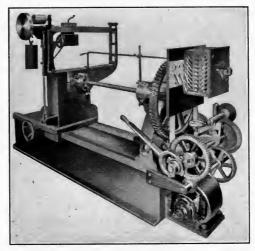
FIG. 33.—Olsen machine for making tortion tests.
