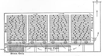
FIG. 70.—A scheme for a radiator kiln.
