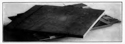
FIG. 85.—Portion of three-ply panel.
