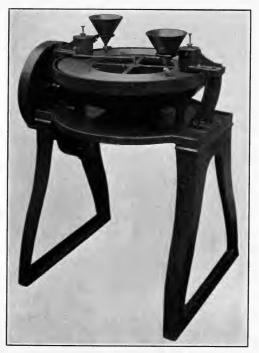
FIG. 39.—Dorry machine for making abrasion tests.
