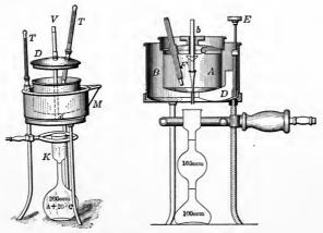
FIG. 86.—Engler's viscosimeter.
