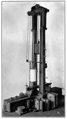
FIG. 38.—Turner impact testing machine.
