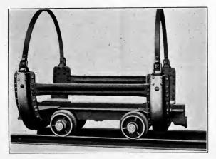
FIG. 78.—Pressed-steel car for cylinder-treatment of ties.<sup>1</sup>
