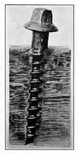
· FIG. 35.—Displacement caused by screw spike. Photograph, Spencer Otis Company.
