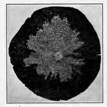
FIG. 73.—Cross-section of pole, showing penetration of creosote.
