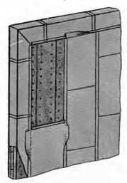
FIG. 45.—Corner of tin-clad fire door.
