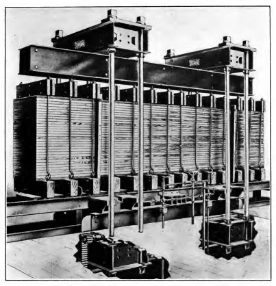
FIG. 83.—Large double-cylinder veneer press.<sup>1</sup>
