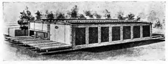
FIG. 68.-A kiln for drying wood.
