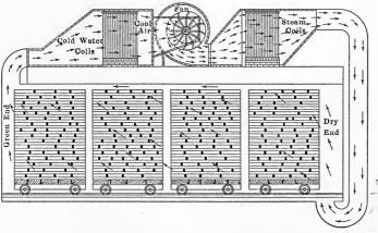
FIG. 71.—A scheme for a blower kiln.
