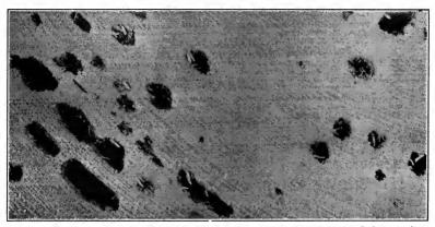
FIG. 44.—Section of wood cut from cypress after attack by wood-destroying fungus (Dædalea vorax).
