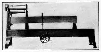
FIG. 31.—Machine for testing light wooden beams.<sup>1</sup>
