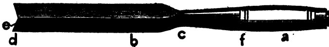
FIG. 25. — Corner chisel. a , handle; b , blade; c , shank; d , bevel; e , cutting edge; f , socket.
