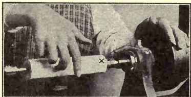
Fig. 10. Stopping the Lathe and Testing the Surface.
