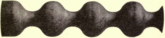
Fig. 50. One-inch Bead and Cove.
