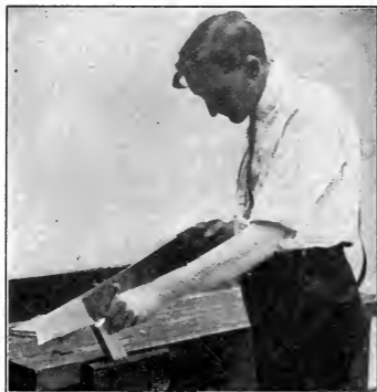
Fig. 72. Ripping Out Waste Material.
