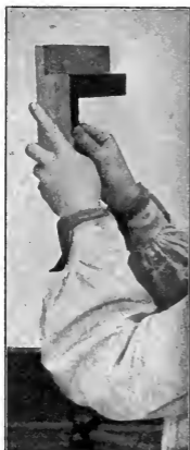
Fig. 57. Testing the Joint. Before the piece has been glued the joint should be placed on the bench and the try-square applied as indicated in this figure.
