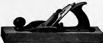
Fig. 167B. Wooden Bottomed Iron Jack Plane.
