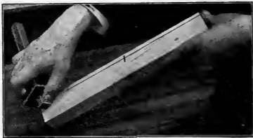
Fig. 16. Finishing a Gauge Line.
