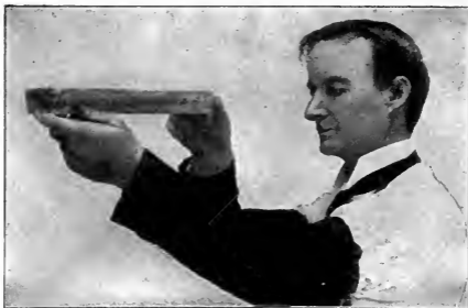
Fig. 2. Sighting for Straightness. Be particular to have the light fall properly upon the piece. Experiment by holding the piece in different positions.
