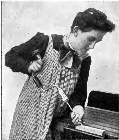
Fig. 71. Setting a Bit to Bore a Hole.
