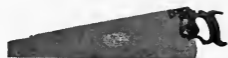
Fig. 178. The common grades of both hand saws and rip saws are made this shape.
