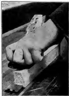
Fig. 6. Jointing an Edge. The plane may be moved along either side or along the center.
