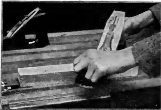
Fig. 9. Swinging the Plane to one Side. This keeps the bit from touching the material on the return stroke.
