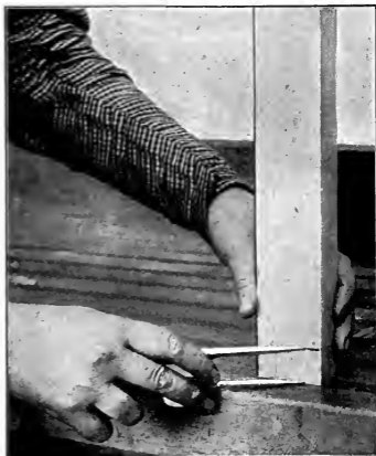
Fig. 105B. Second Step in Locating the Point at Which to Set the Compasses.
