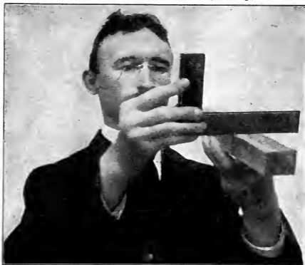
Fig. 3. Testing from Edge to Edge. The try-square may be held either side up, but the beam should not be placed against the edge in making this test. Compare this use of the try-square with that shown in Fig. 12.
