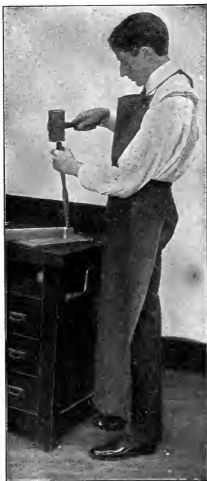
Fig. 52 Splitting out Waste Material. Do not use this method until you have learned to work as shown in Figs. 53A and 53B.
