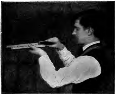
Fig. 54. Testing a Gain with a Chisel.
