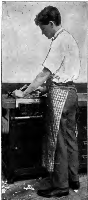
Fig. 31. Jointing an Edge of a Thin Piece. Use the vise only when the piece is too thin to hold against the stop. Except for very light planing you should stand more at the end of the piece than the young man in this picture. Compare this position with that shown in Fig. 1.
