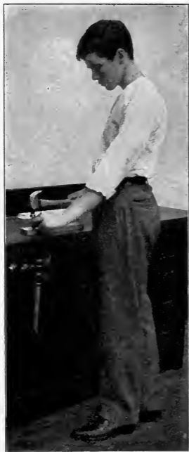
Fig. 25. Starting a Nail. Examine the nail from two positions as in boring (Figs. 35 and 36).
