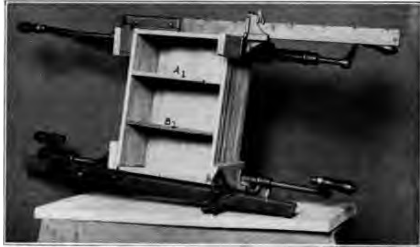
Fig. 286. Gluing Together a Box.
