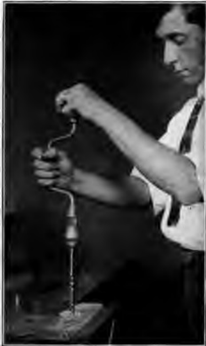
Fig. 137. Using a Try-Square as a Guide in Boring.
