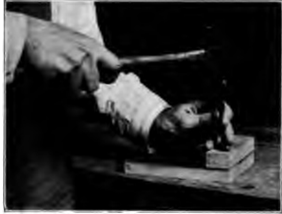
Fig. 165. Using a Nailset
