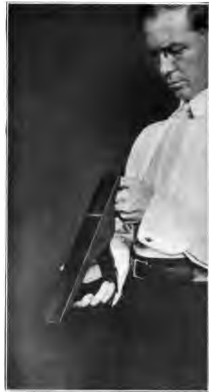
Fig. 102. Sighting Along the Sole of Jack-Plane.
