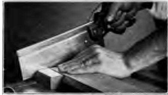
Fig. 90. Using the Back-Saw with Bench-Hook.
