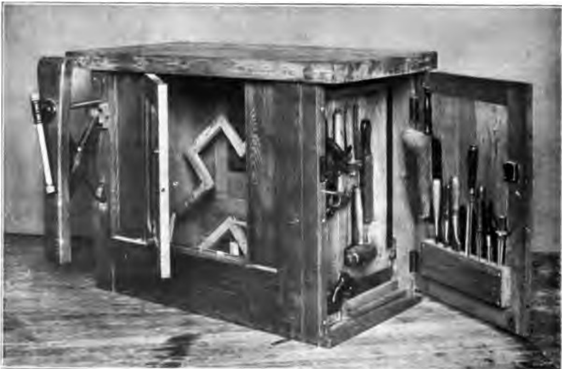
Fig. 167. Woodworking Bench Used at Pratt Institute, Showing Self-Adjusting Upright Vise.
