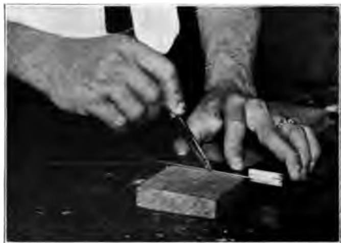
Fig. 204. Scribing with Knife by Try-Square.
