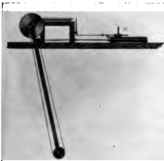
Fig. 48. Cut-off-Saw. This saw trims the ends of timbers.
