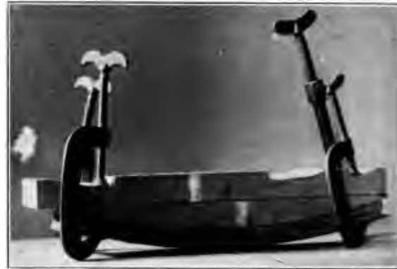
Fig. 299. Bending Boards into Shape after Boiling Them.
