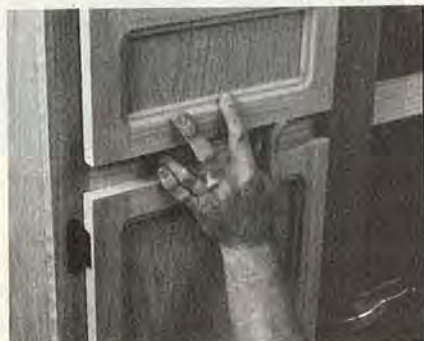
Positioning the drawer front
