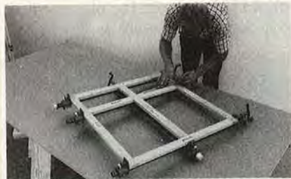
Marking dowel pin locations
