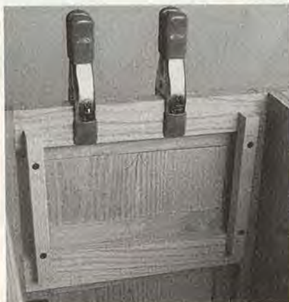
Attaching false front with cleats
