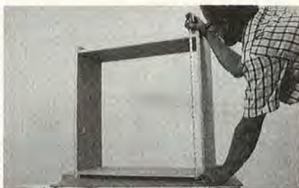
Measuring height of divider
