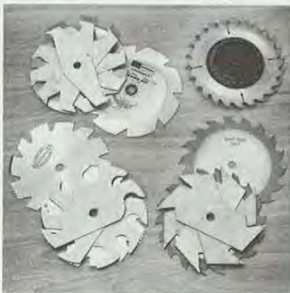
Types of available dado tools. Clockwise from lower left: a flat-ground steel dado stack set with interchangeable outside cutters and 5 chippers; a thin-rimmed steel stack set; a carbide-tipped steel adjustable dado blade; a carbide-tipped steel stack set.
