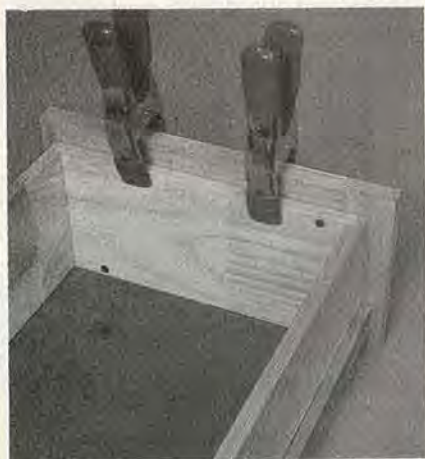
Screwing front to drawer
