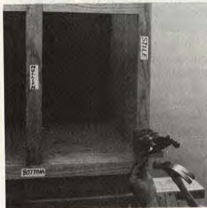
Attaching the face frame
