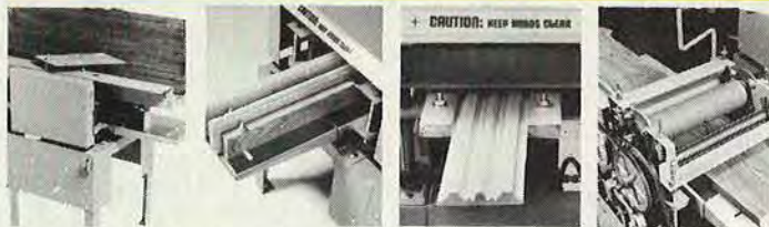
Jointer attaches in seconds ... designed to let you move directly to planing without changeover.
