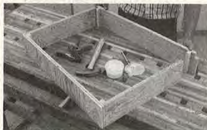
Assembling the cabinet's base
