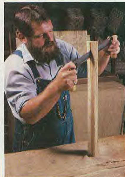
Splitting the billet with a drawknife
