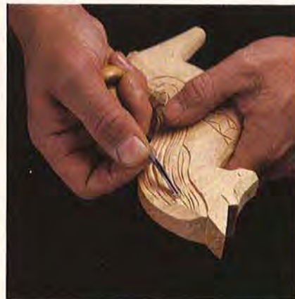
Incising lines using the V-tool
