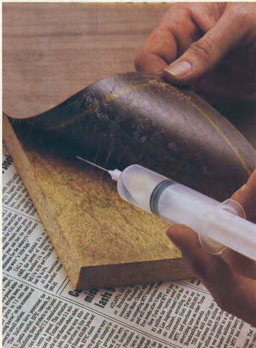
Using refinisher to release the bond
