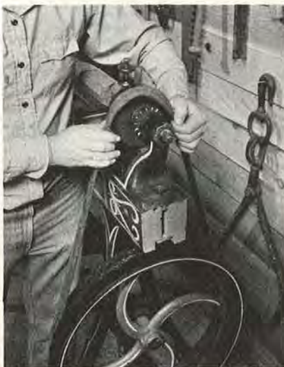
Some Barnes' machines, like this lathe, used a perforated leather belt to transfer power from the foot pedals.
