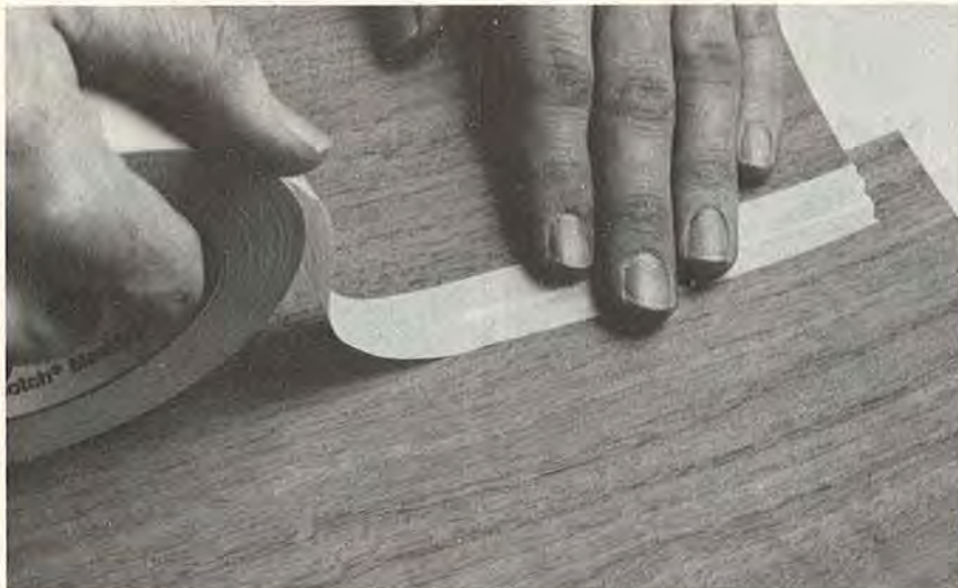
Overlapping veneer with irregular edges
