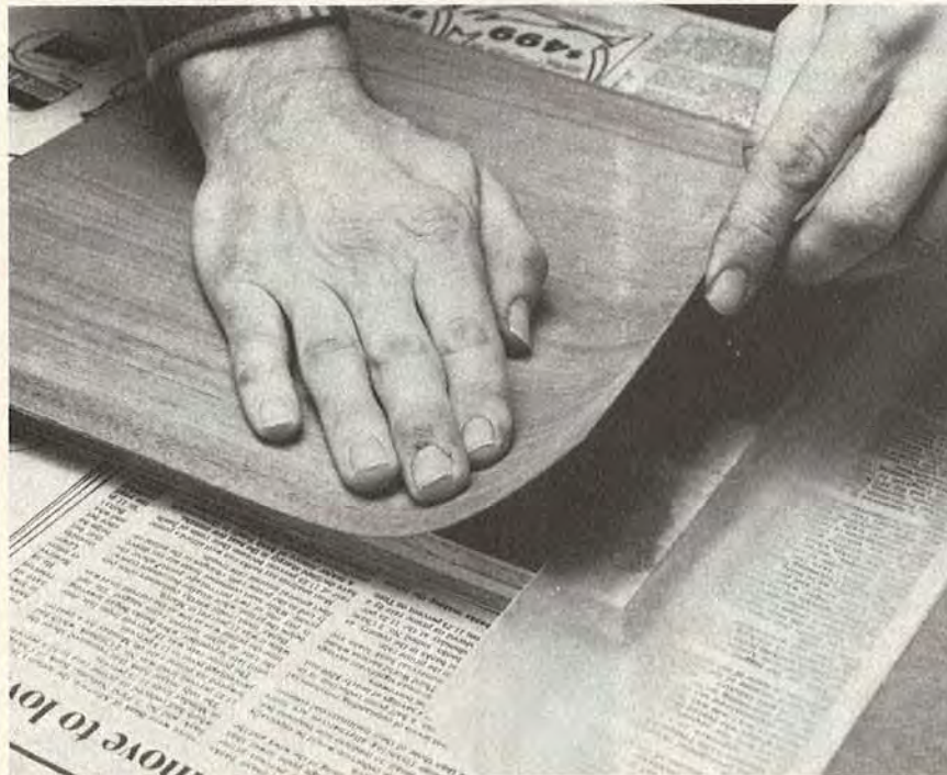
Pressing the veneer from side to side
