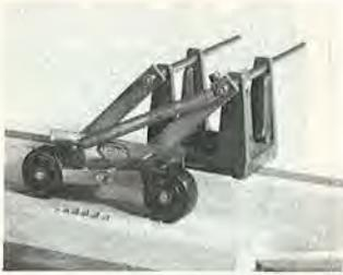
The RIPSTRATE has revolutionized ripping on table and radial arm saws by keeping hands away from the blade. Holds work firmly against the fence and prevents kickbacks. Self adjusting. Over 10,000 in use by amateurs, professionals, schools, government and military installations. \$66. Check, Visa, M/C. Call toll free 1-800-421-0256. Free brochure. FISHER HILL PRODUCTS, 4A Fisher Hill, Fitzwilliam, NH 03447.
