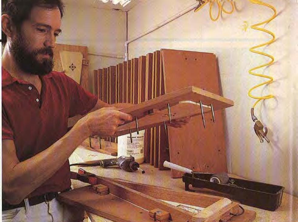
Gene assembles the instrument body by mounting the top, sides, and back in a two-piece clamping fixture. He spreads Titebond on the parts with a small paint roller, then bolts the halves together.
