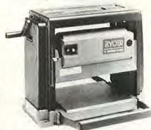
A brand new planer, the AP-10, but dubbed the "Plane Jane" by Ryobi, weighs only 58 pounds and measures 19 $\frac{1}{4}$ "L x 16 $\frac{3}{4}$ "W x 14 $\frac{1}{4}$ "H. Planes material up to 10" wide and 5" thick and features all-ball bearing construction and externally accessible brushes. Standard accessories include 10" blades, a blade adjustment gauge, adjustment tools, extension rollers and owner's manual. \$659. RYOBI AMERICA CORP., 1158 Tower Ln., Bensenville, IL 60106, 312-766-1621.
