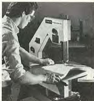
The Delta 16" motorized band saw features an innovative three-wheel design that delivers high capacity 16" blade-to-frame and 8" depth of cut capabilities. Features include: C-type cast-iron frame, adjustable 16" x 16" cast-iron table that tilts to 45°, ball bearing supported blade guides, blade tension scale, rip fence and miter gauge, removable safety switch. DELTA INTERNATIONAL MACHINERY CORP., 246 Alpha Drive, Pittsburgh, PA 15238. Call toll-free: 800-438-2486. In PA, 800-438-2487.
