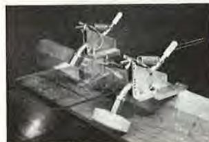
SHOPHELPER™ SAFETY GUIDES, a totally interchangeable system for controlling stock on saws, shapers and other stationary tools. Single direction bearings guard against kickback and provide smooth, even cutting. Additional mounting brackets allow quick easy interchangeability of guides on machinery. Set, complete with brackets, \$79.50. See your local dealer or call: 800-828-8833.
