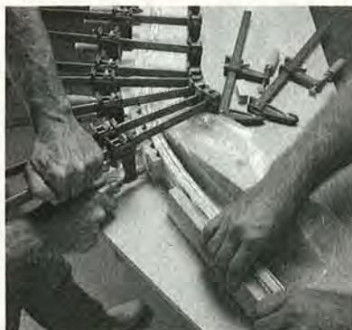
the center marks on the form and the strips line up. (We poured the glue into a paint tray and applied it to the strips with a narrow paint roller. We also found it handy to have a helper on hand when bending the wood around the curves.)
