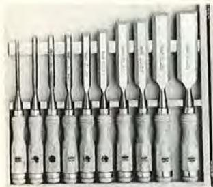
FREUD 10 piece chisel set— $\frac{1}{4}$ " to  $1\frac{1}{2}$ " of premium chrome vanadium steel. Hardness of 58-60 Rc. The most tool for the money. Boxwood wooden handles bound by double-steel hoops for strength and durability. Packaged in a fitted box-jointed wooden case. \$50.00 includes s/h. BRADY SUPPLY CORP., P.O. Box 326, Elmira, NY 14902.
