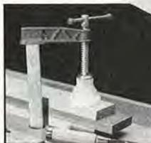
**HOLD-DOWN CLAMP** Use it on the benchtop or in the slotted "deadman" leg to secure oversize pieces horizontally or vertically. Pivoting nylon pad grips almost any shape piece firmly.
