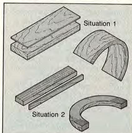
would want to slice strips from one of the faces of the board. But in situation 2, for the greatest strength you should rip material from one of the board's edges.
