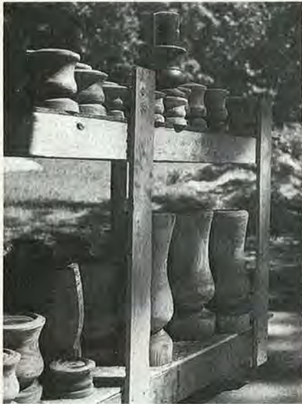
Elm, dense and hard, supposedly is tough to PEG-treat. Here, elm turnings of thick, thicker, and thickest stock await finishing.
