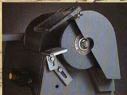
Grinder with tool rest and guard
