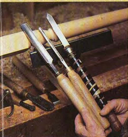
A large gouge, small gouge, and a modified parting tool that can act as a skew are the only tools Bert really needs for between-centers turning.
