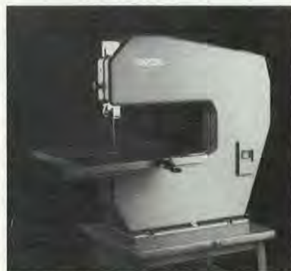
INCA Professional 20" Bandsaw carries a blade range from 1/16" to 1"
