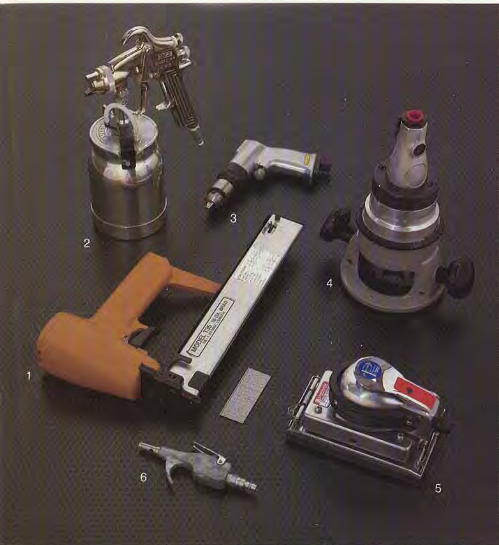
Air tools, a woodworking option. Shown above: 1) Bostich brad tacker , requires 4.7 c.f.m. at 80 p.s.i. for 100 nails per minute, $435; 2) Binks production spray gun , 6.5 c.f.m. at 40 p.s.i., $90; 3) Allied Pneumatic 1/8" air drill , 4 c.f.m. at 90 p.s.i., $60; 4) Rockwell industrial router , a hungry 50 c.f.m. at 90 p.s.i., $750; 5) Powerdyne orbital sander , 6 c.f.m. at 60 p.s.i., $30; 6) Speedaire blower , all pressures, $5.
