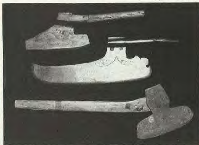
Top. Standard goosewing ax with elongated eye, slight poll, and sound old handle; thought to be German, c. 1800. Middle. Exceptional Austrian goosewing with 20 1/2° bit and decoration, c. 1700. Bottom. Typical American "broad ax" with bent handle, c. 1840.
