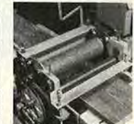
Optional sanding head converts planer to power-feed drum sander!
