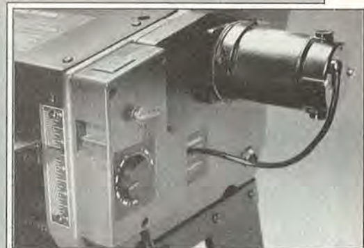
Small, separate gear motors with electronic controls make the Shopsmith (shown) and Woodmaster the only machines with variable feed.
