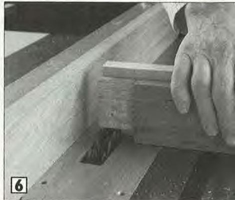
6 Using the same notch-and-test method, cut the tenon setback.
