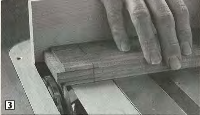
3 With a 3/4" dado set, test-notch the tenon cheek.
