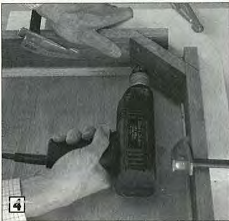
4 Glue the block ends, then drill the pilot holes and drive the screws.
