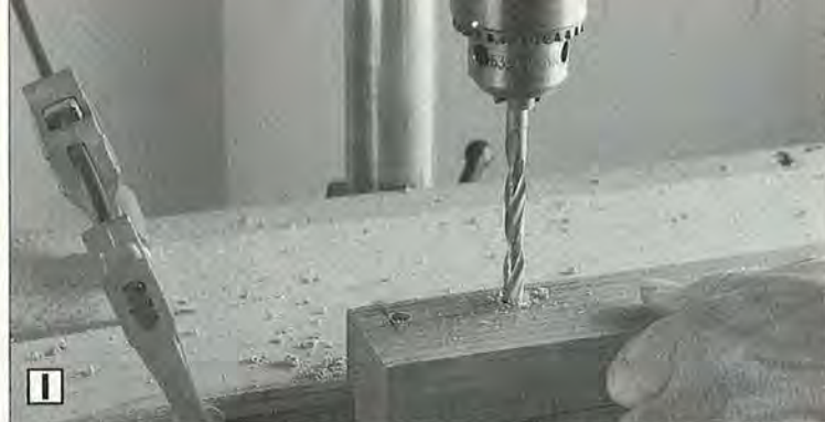
1 To make the mortise, drill a series of holes to the desired depth.
