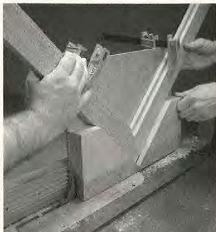
Cutting the spline groove with a V-block jig and helper.
