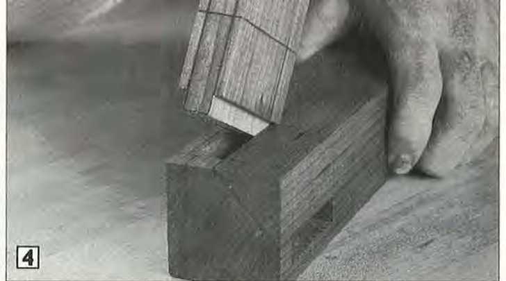
4 Test-fit the tenon in the mortise; adjust the dado height, if necessary.
