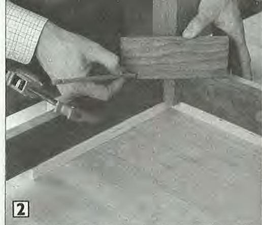
2 Align the corner block with the marks on the rails, then mark block for finished length.
