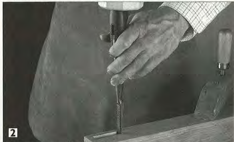
2 Square up the mortise with chisels. First, use a narrow chisel to make stop cuts as shown, then a wide chisel for the sidewalls.
