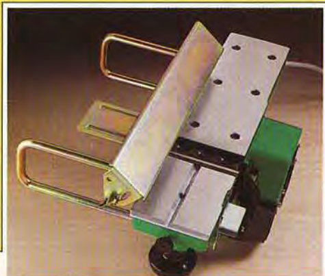
Left: The longer the fence, the more accurately a power planer will joint edges. We like the extra-long fence on the Hitachi F-30A, which also tilts for bevel cuts.
