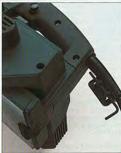
A flip-down foot on the Metabo 0882 keeps the spinning knives from hitting your bench when you set down the tool. A holder on the cord keeps the tool's Allen wrench handy for changing knives.
