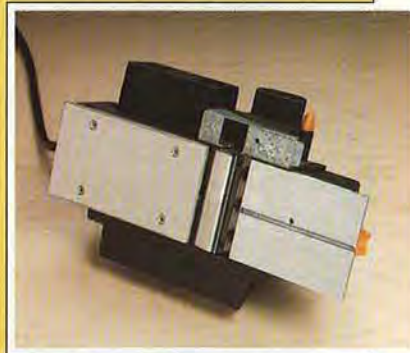
Left: The center-balanced handle design of the Hitachi F-20A at left, is typical of planers designed for one-handed operation. You can also use it with both hands. The handle on the larger F-30A at right, requires both hands for operation.
