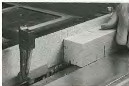
Cutting a kerf in the top end of the table leg on the table saw.
