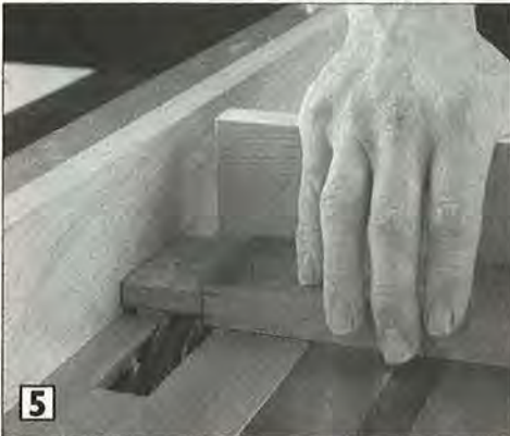
5 Cut the tenon cheeks, working from the tenon shoulder to the end.
