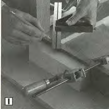
1 Place leg and rails in the jig, then mark the corner-block location on the rails.
