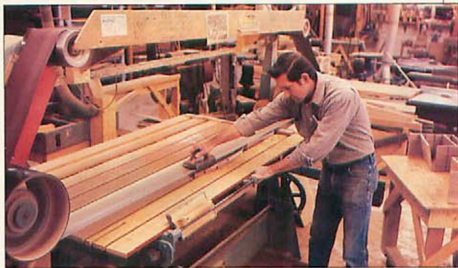
At the stroke sander, Ron Haldy smooths a rocker part. The 6"-wide, 288" belt of 60-grit abrasive sands at a touch of the pad. This is the only sanding done to most parts before the finish goes on.
