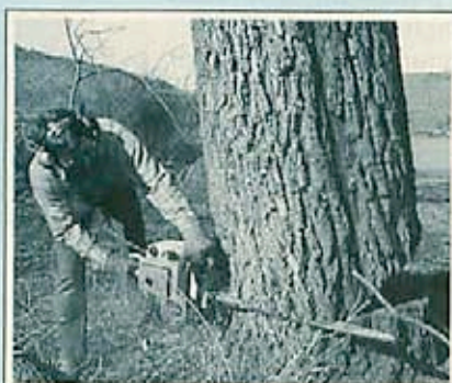
A backcut fells the tree as a winch provides a powerful pull opposite lean.
