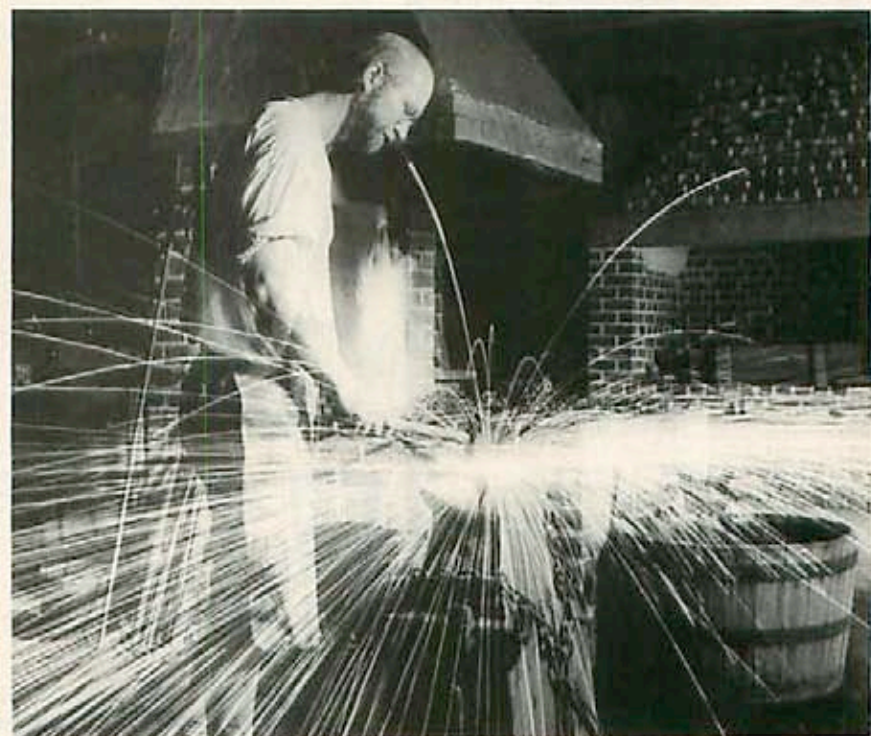
Hot flux of melted sand or borax splatters as blacksmith Rick Guthrie welds the steel bit into the iron axhead.
