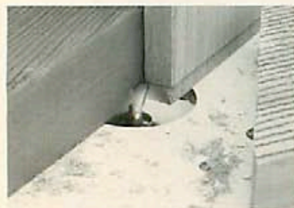
Routing a dovetail pin along one end of a drawer shelf
