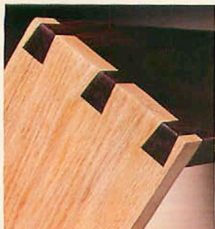
Leigh, Omnijig, and Keller make through dovetails. We used the Keller 24" jig to make this one.
