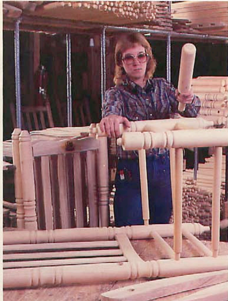
Jeri Colley brushes on a slow-drying casein glue, then assembles the pieces with the help of an ash mallet. Because of the 1/2" depth of the holes and close tolerances, she uses no clamps.
