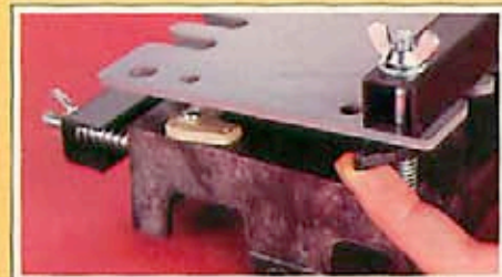
A ratcheted tab adjusts the template in \frac{1}{64} " increments for easy setup.
