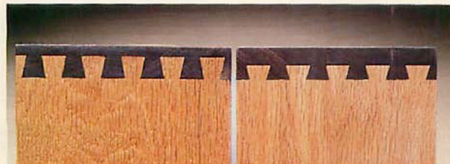
A bit of a difference: \frac{1}{2} " dovetail joints made with Black & Decker's dovetail bit and jig ( left ) and Sears' bit and jig ( right ).
