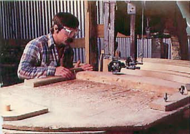
A large plywood jig, secured by a dowel, guides the sawing of the rocker. The jig holds the stock and moves through the cut in a circular motion.
