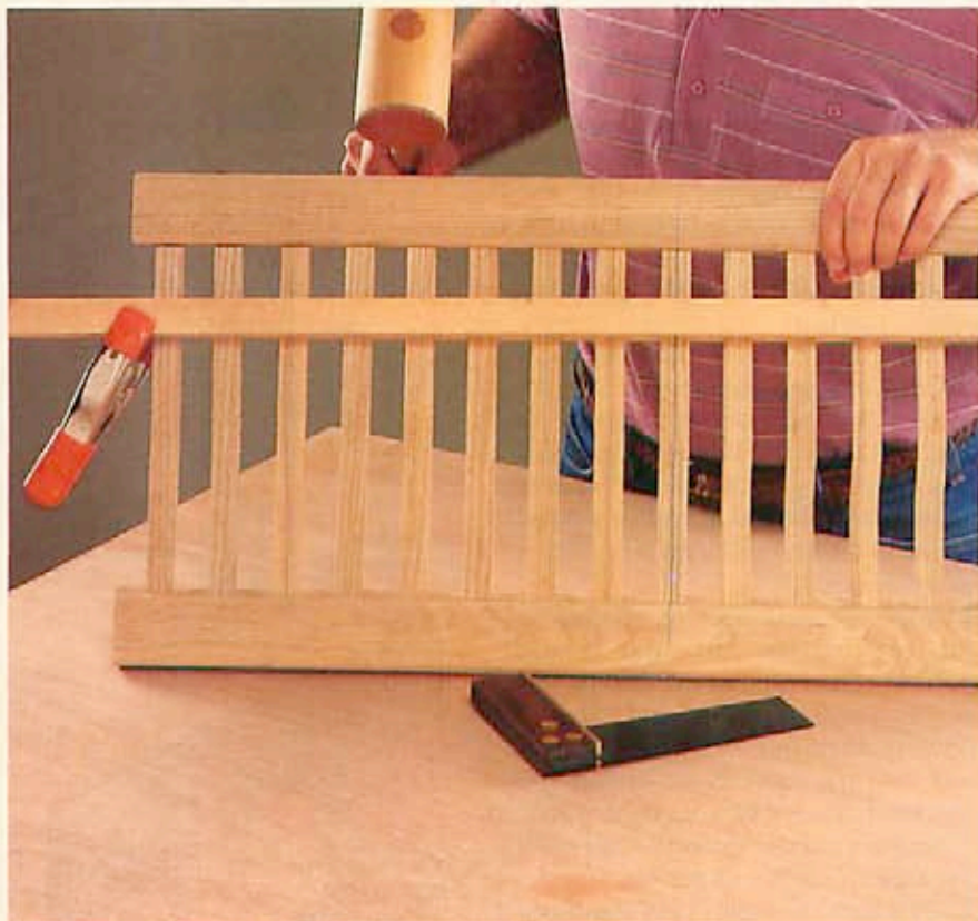
Align the top rail with the marked middle slat, and then fit the rest of the ash slats into the groove in the top rail.
