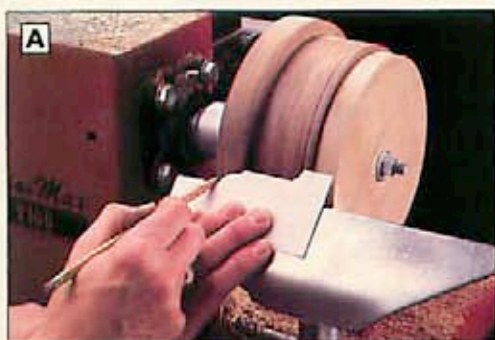
Mark profile lines on teak lamination with the lathe running.
