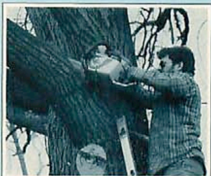
Limbing with an undercut and an overcut prevents splitting wood.
