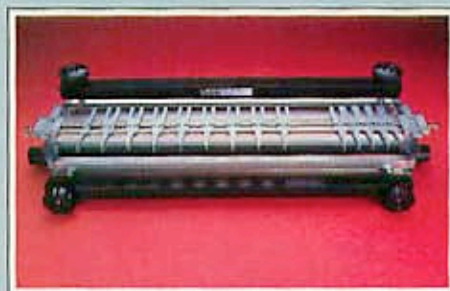
Adjustable guide forks on the Leigh jigs enable you to vary the size and spacing of the pins and tails. This jig makes half-blind dovetails and through dovetails. Both 12" and 24" versions are available. The jig comes with an excellent owner's manual.
