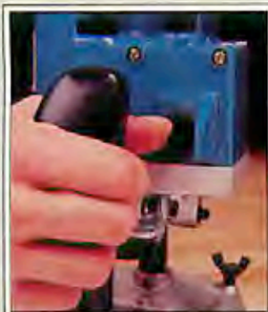
Exposed toggle switch can get turned on by accident, even while the router isn't being used.
