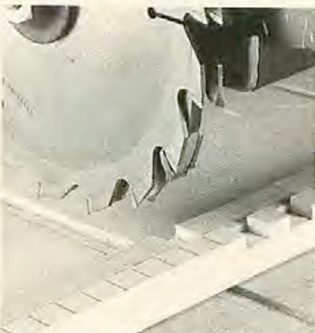
Align the marked dado lines on the maple with the dado cut in the fence.
