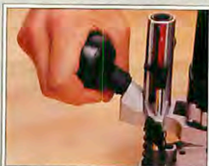
Twist knob (right-hand handle) locks easily, but may loosen while you're routing or handling the router.
