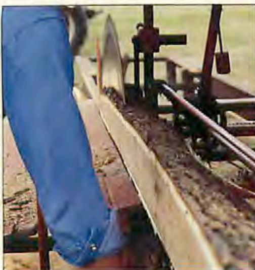
Darrell controls throttle and feed rate as the sawblade bites into the "dog board," the last full-thickness board cut off a log. He saws each board to \frac{1}{16} " thick.
