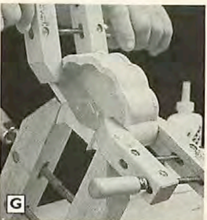
Hand screws make clamping the base back onto the box body easy.
