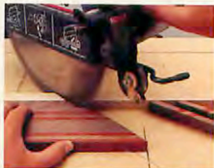
Mark a stop line on the table for consistent lamination lengths. Miter the handle pieces on the radial arm saw.
