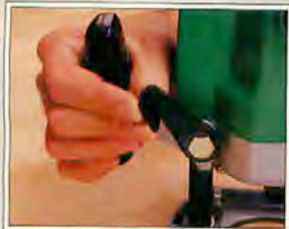
Manual locking lever requires the most effort to operate. Push down with thumb to lock; up to unlock.
