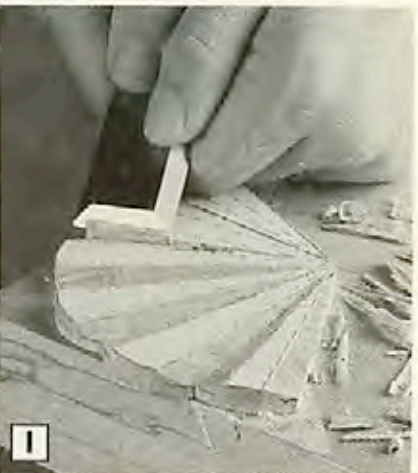
Sculpt the lid top to rough shape with a sharp 1\frac{1}{4} " chisel.
