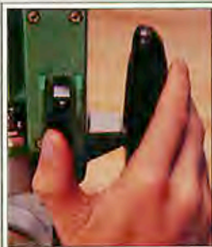
On the Hitachi TR-12, you have to let go of the right-hand handle to actuate the rocker switch.
