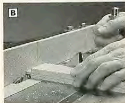
Use a miter gauge and auxiliary wood fence when cutting the stub tenons.
