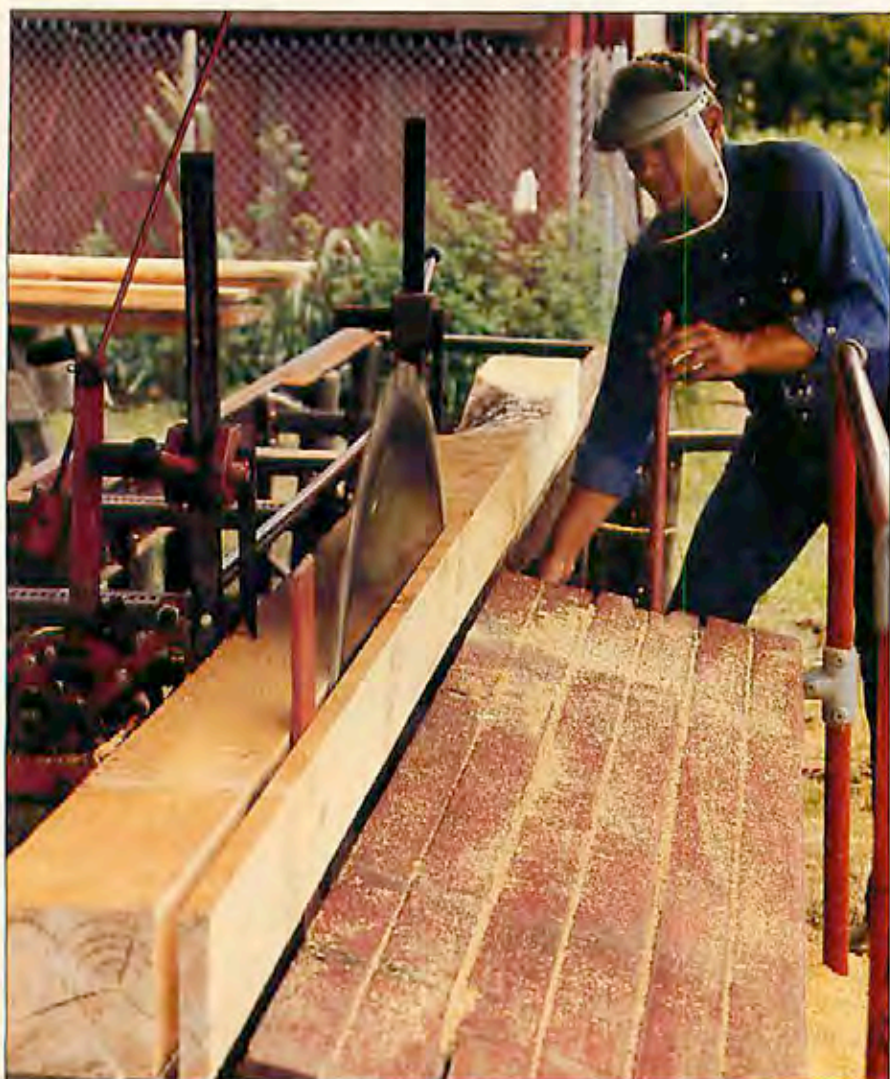
With a one-man, backyard sawmill, Darrell Mattson rips wood for his woodworking projects as well as nominal-size boards for construction.
