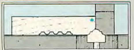
Make the final cut with a \frac{3}{4} " classical bit, centered on front edge of fence, as shown on the drawing.
