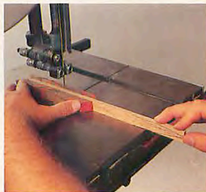
Cut the letter opener handle and blade to shape on a band saw fitted with a fine-tooth blade.
