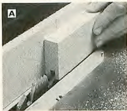
Cut the \frac{3}{8} "-deep groove with a \frac{1}{4} " dado blade on the table saw.
