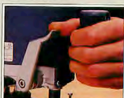
Spring-actuated lever automatically locks when you release your thumb. We found this type the easiest to use.
