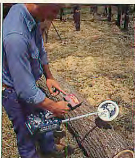
Without a metal detector, a home sawyer takes the chance of hitting metal embedded in the log. This model reads right through a log.
