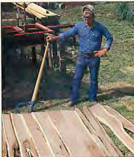
A half hour's sawing yields several board feet of black walnut. Darrell turned the log in order to obtain a few crotch-figured boards he'll save for special projects.
