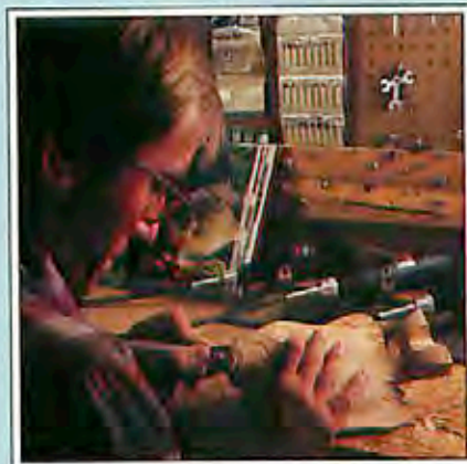
A flexible-shaft Moto-Tool, one of five such tools Rick uses, bites into the cherry of a bluegill's lips.
