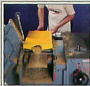
2 After swinging the jointer tables out of the way, he surfaces the stock to exact thickness on the thicknesser.
