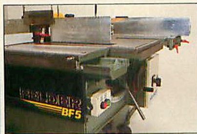
Above: Tilting-arbor shaper is a Felder exclusive; rip fence for table saw slides to far side of jointer table, providing a 39" rip capacity. Right: Felder BF5/41: Largest and most expensive machines.
