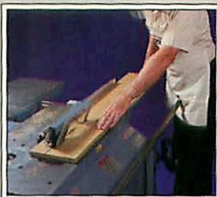
3 With the jointed edge against the saw fence, Ray rips the stock to the desired width on the table saw.
