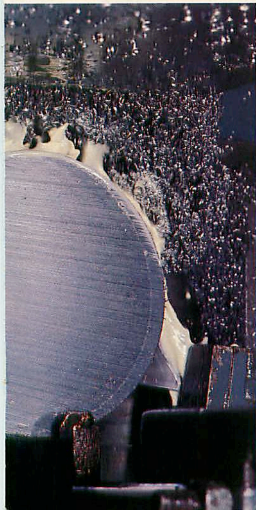
Left: A saw blade begins as part of a rolled steel bar that weighs 1,200 pounds. A liquid-cooled band-saw blade slices the blanks.
