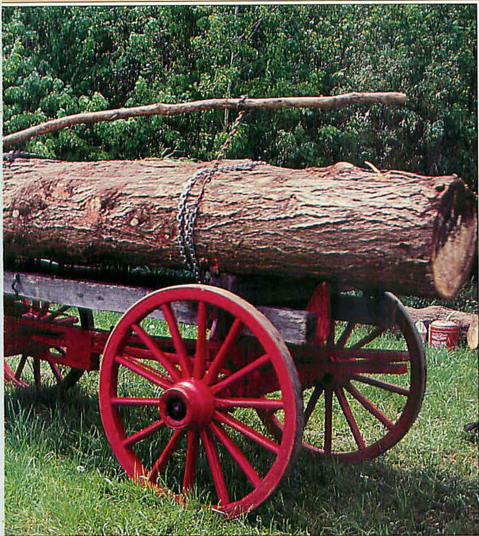
Above: Chains and a levered hickory sapling hold the huge hemlock logs in place on the wagon. A fully loaded wagon would have six or more logs and could weigh upwards of 10 tons. Hilary's wagon dates to about 1900.
