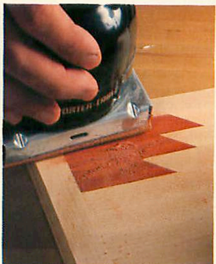
If your project consists of two or more wood species, use this method: Force glue into the cracks with a plastic putty knife ( left ). Then, run a palm sander over the glue lines to force sawdust into them ( right ).
