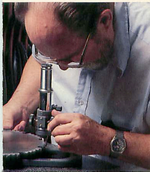
Above: Peering into a 100-power microscope, Leo makes the final inspection. He checks for microscopic cracks in the brazed joints.
