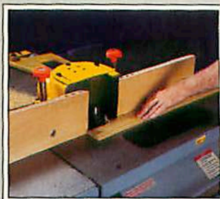
4 Ray forms his oak molding on the shaper. For clarity, we've removed the front guard on the shaper.
