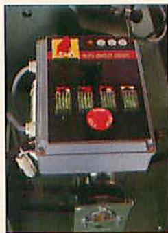
Left: Kity K5: To switch functions on this inexpensive, one-motor machine, you change the drive belt from one component to another. Right: Kity DD: You can begin with the basic drive unit and one or two machines, then add the rest as need and budget allows. Center: Central control panel on the Kity DD operates electric clutch (at bottom of photo) to switch functions.
