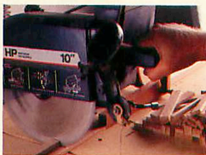
To cut pieces to identical lengths, clamp a stop to the fence of your radial arm saw or power miter saw.
