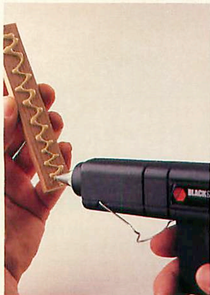
Apply a wavy line of hot-melt glue to the back of the onlay piece.
