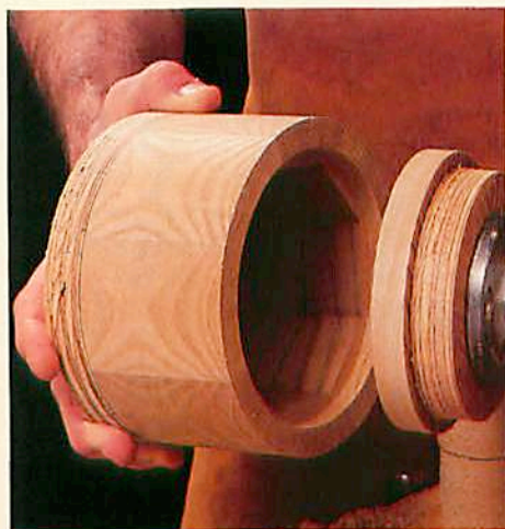
Periodically check for a snug-fitting bottom while turning.
