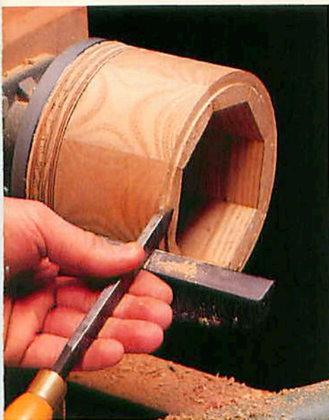
Periodically check for a snug-fitting bottom while turning.
