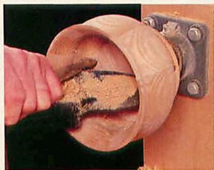
For turning the sidewall, we had good results using a bowl scraper, and we smoothed the bottom with a skew.
