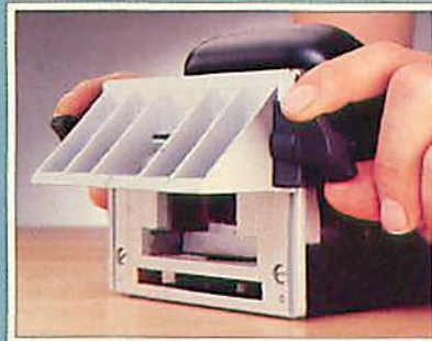
The Freud JS100 fence features quick-action adjusting knobs.
