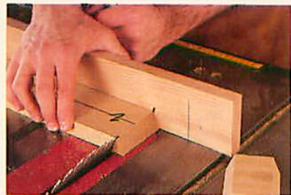
Now, flip the board over again and make another cut to reestablish the bevel angle. Repeat this process.
