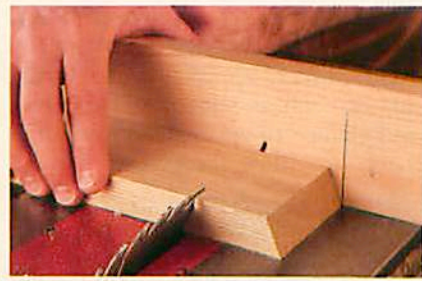
For bowls with horizontal grain, make your first bevel-cut, mark a cutoff line on the auxiliary fence, flip the board over, and make the second cut.
