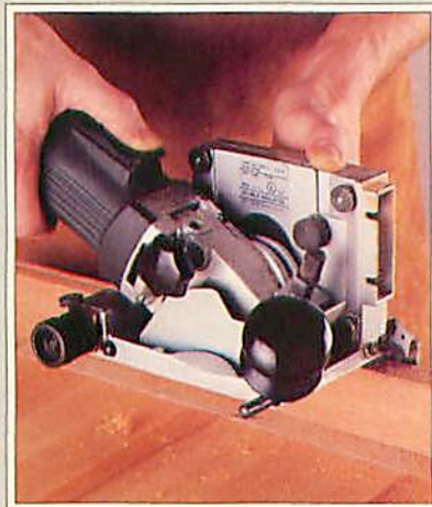
To cut with the Elu, you must simultaneously raise the handle and hold the Elu against the stock.
