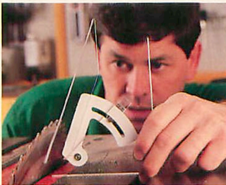
With an adjustable triangle, set the blade angle carefully.
