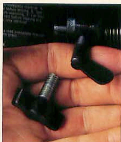
Most of the machines have plastic locking knobs, left , to tighten depth stops and belts. The flipper lever used on some Sears and Black & Decker machines, right , should give more service.
