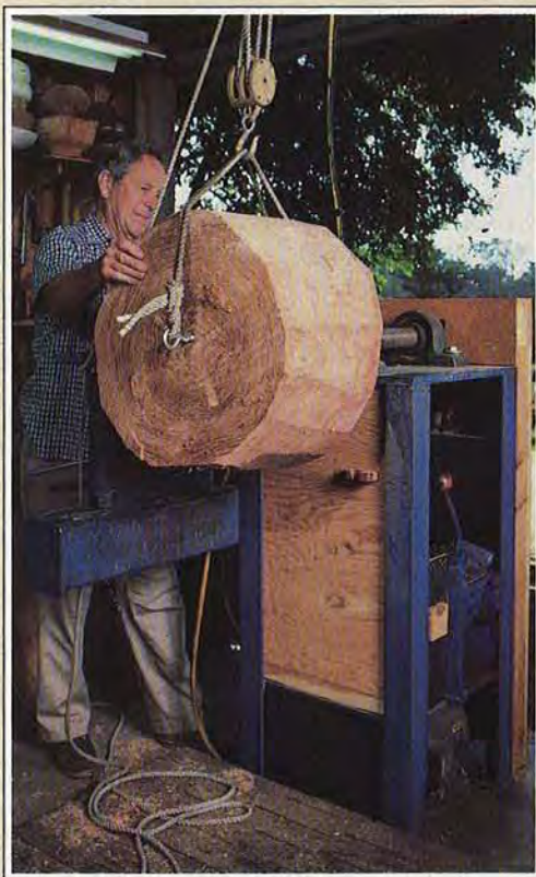
▲ A block and tackle is a standard tool when 150-pound bowl blanks aren't uncommon around the shop.
