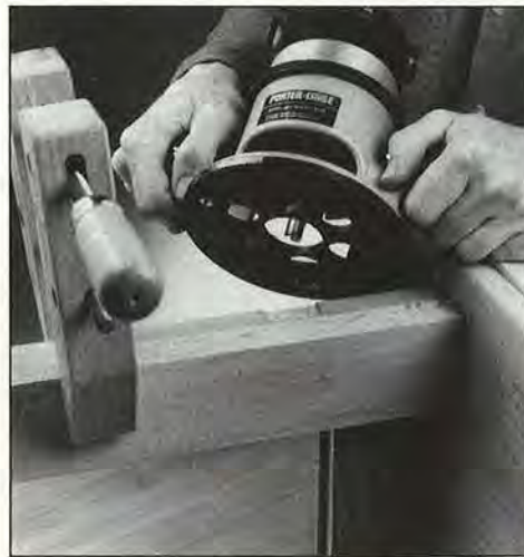
Clamp a piece of scrapwood to the front of the side frames for additional support, and rout the hinge mortises.
