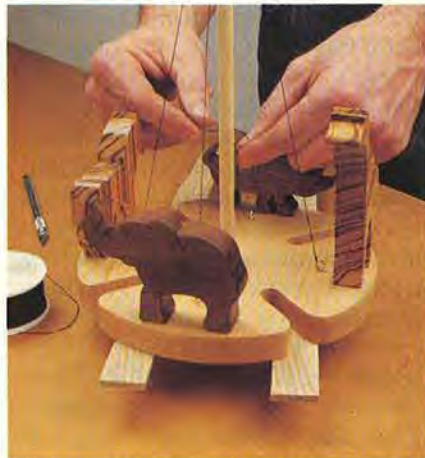
Support the platform on the base with scrap spacers. Hang the platform from the center dowel.
