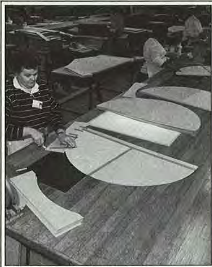
Assembling an intricate veneer pattern can require up to 80 separate steps.
