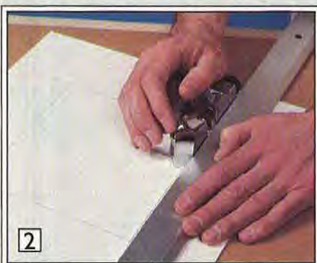
▲ With the straightedge held down firmly, push the mat cutter alongside it to cut the mat opening.
