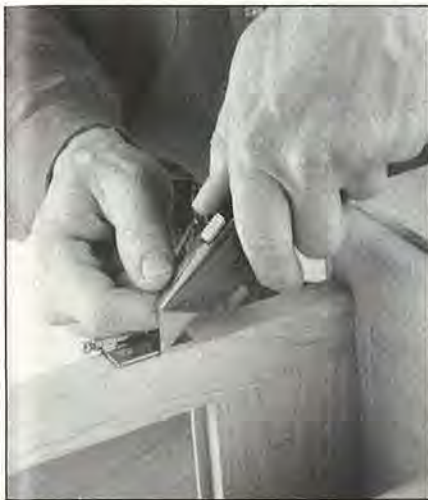
Screw the hinges to the cabinet. Next, scribe the hinge locations into the front of the side frame.
