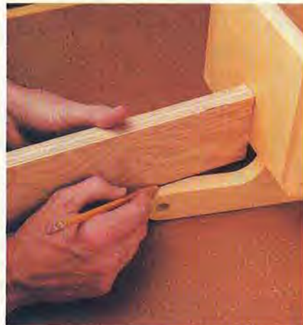
Mark the wheel opening on the top edge of the handle fronts.
