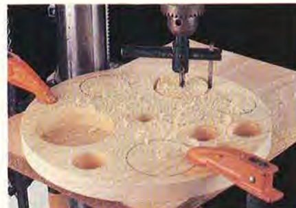
We used a circle cutter for cutting the larger-diameter holes.
