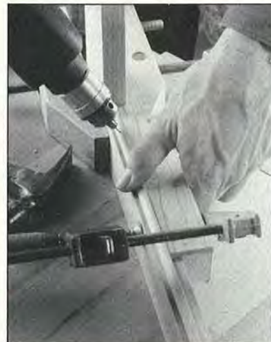
Use the jig to position the glass stops. Then, drill pilot holes and brad the stops into place.
