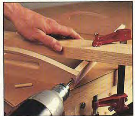
Clamp the tray frame to a work surface, and drill the \frac{1}{4} " dowel holes.
