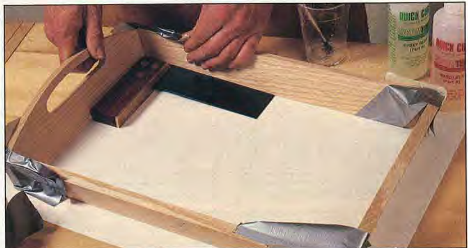
Tape the epoxied corner joints together tightly. Check that the bottom edges are flush and that the tray frame is square.
