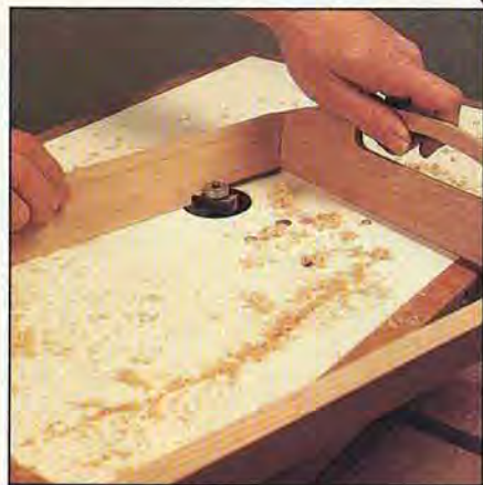
Rout a \frac{1}{4} " rabbet \frac{1}{4} " deep along the bottom inside edge of the frame.
