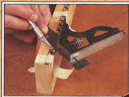
To miter the banding, align it and a combination square with the edge of a piece of scrap stock, and follow the square's blade with an X-acto knife.
