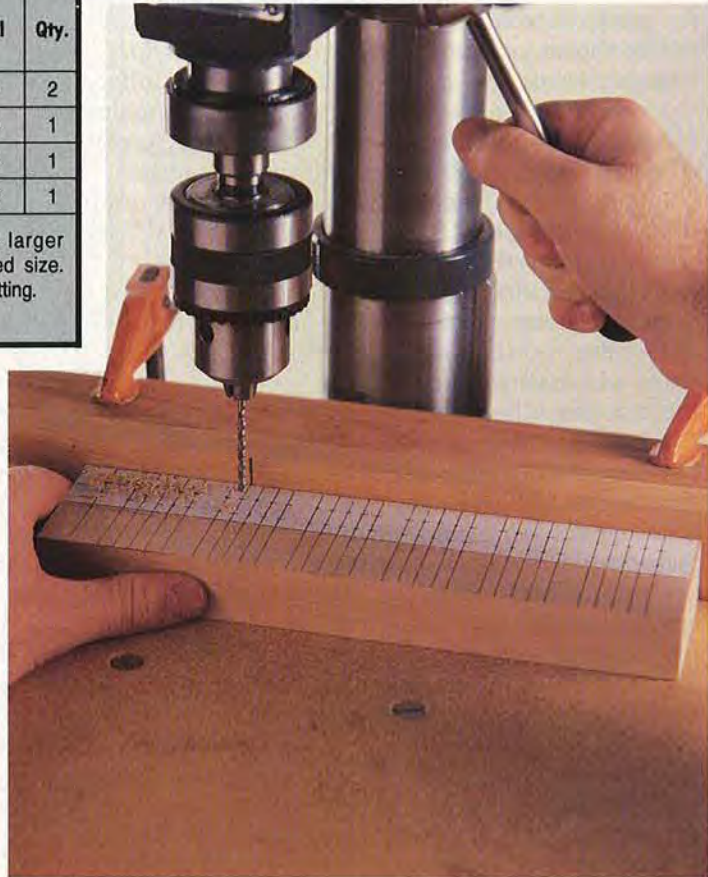
Use the fence and marked lines to drill evenly spaced player holes in straight rows.
