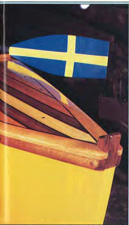
▲ The wherrie's deck sports poplar, teak, vertical-grain Douglas fir, and Sitka spruce. To allow for movement, Art filled between each plank with caulk. His oars carry Sweden's national colors.
