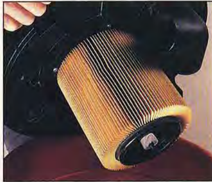
Because of greater surface area, pleated cartridges won't clog from fine dust as quickly as foam and paper filters.
