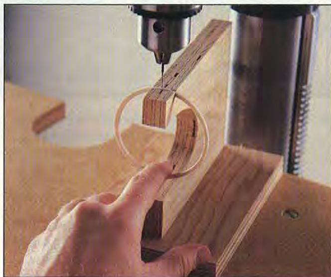
With a sharpened 4d finish nail and a drilling jig, drill a hole through each birch plywood ring.
