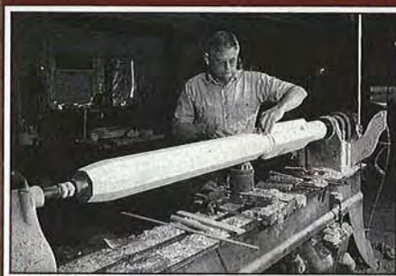
▲ This 8' bedpost almost fills the 9' lathe bed. George sands concave areas with a sandpaper-wrapped dowel.
