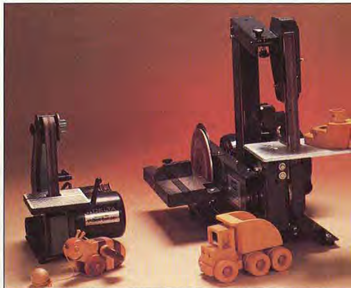
▲ These benchtop machines serve the small-project maker. From left: Delta model 31-050 strip sander, AMT model 4150 strip/disc sander, and the Delta model 31-460 belt/disc sander.
