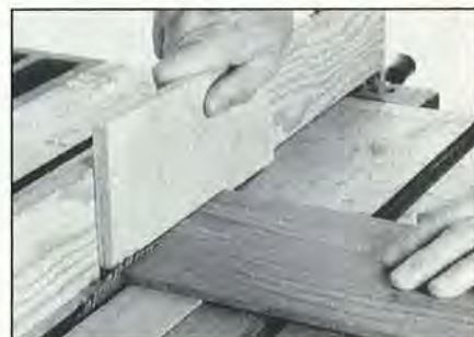
For safety, use a thin push block when cutting to length the narrow block-pattern pieces.
