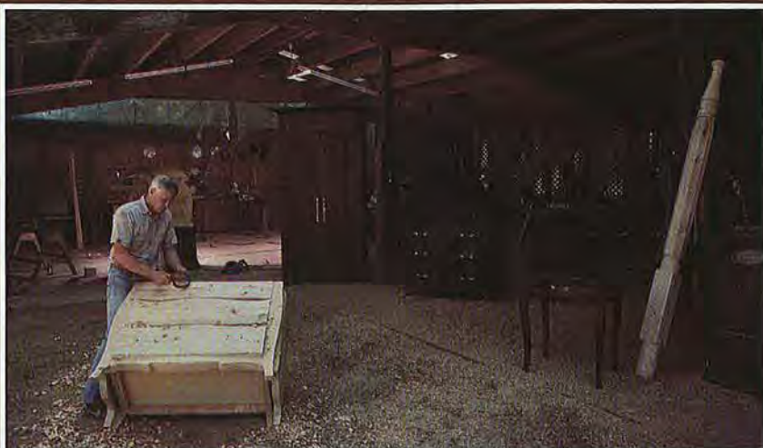
▲ In Louisiana's climate, George often chooses to bring work out in the sunshine. To shape the bombé chest, George takes off cypress with an "in-shave" or scorp. Under his attack, the chips really fly.
