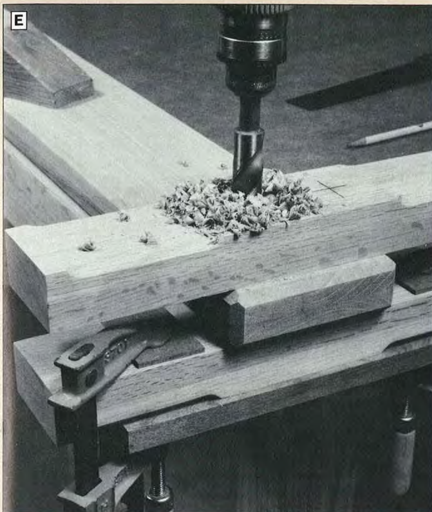
E Mark the centerpoints and bore a pair of \frac{3}{4} " holes through the upright-stretcher rail assembly, backing the stock to prevent chip-out.
