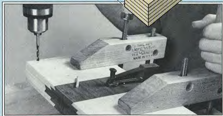
After marking reference lines 6" from the marked centerline, drill two guide-
