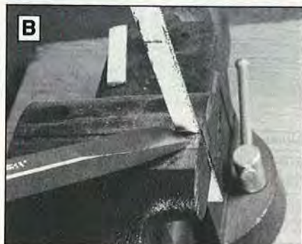
B Scribe marks every 2\frac{1}{2} " on the hacksaw blade. Then, shear scraper blades to length with a cold chisel.
