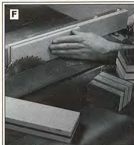
With the power OFF, set the rip fence to the height of one segment, test the setting with a scrap piece, and then ...
