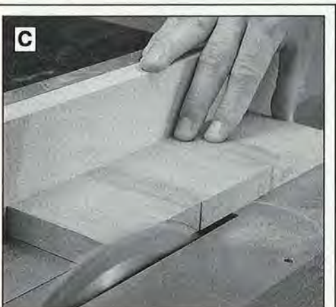
... take off a minimum amount of stock on both sides with your tablesaw to square the segment.
