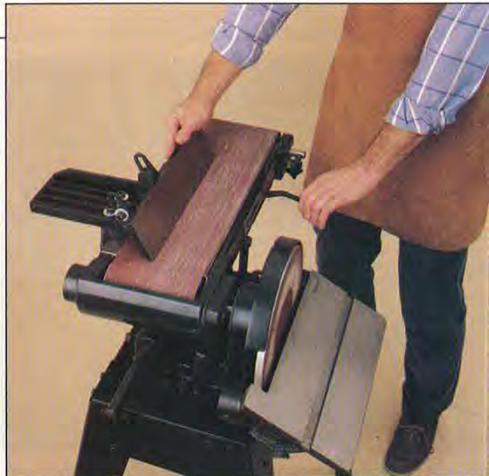
Convenience features and an edge-sanding fence make the DeWalt model 1765 stand out from the crowd.
