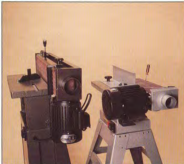
▲ The Foley-Belsaw 6×89" model 4130901 on the left and its near-twin, the Total Shop 6×48" model 943 on the right, operate as horizontal or edge sanders. Both units have the miter gauge shown on the Foley-Belsaw and the fence mounted on the Total Shop.
