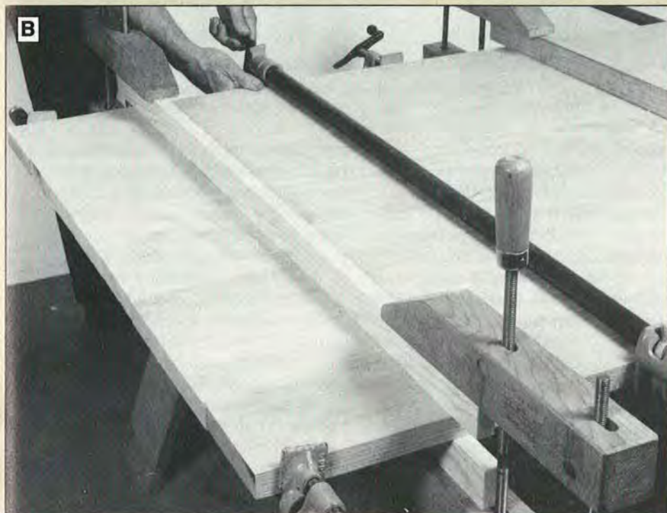
Glue, spline, and clamp the two tabletop halves together, clamping long scrap pieces to the top and bottom to ensure flatness.
