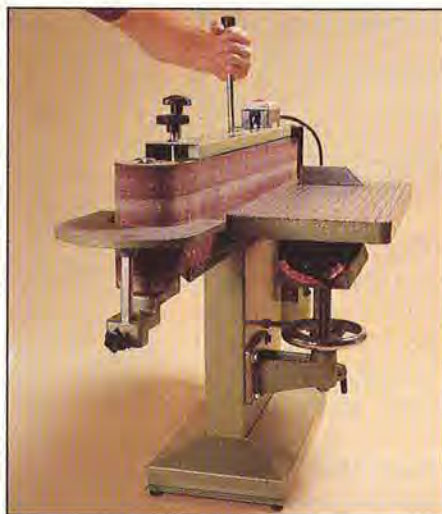
A locking lever atop the Grizzly model G1531 edge sander loosens the tension on the belt in a snap. Elevating tables help you use the belt's full surface.
