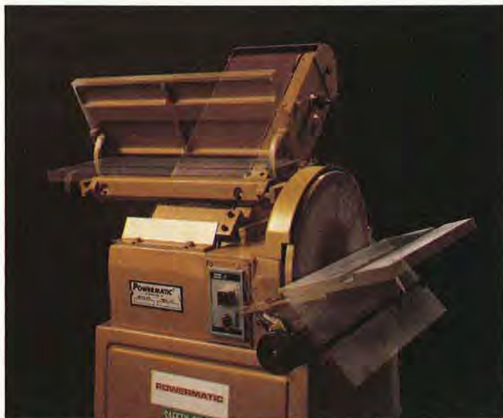
You can release, tilt, and lock the tables on the Powermatic 30B by turning one large knob on each end of the tables.
