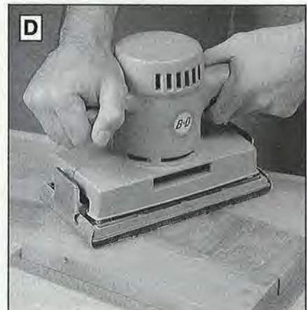
To hold the layers in place while you sand them, lay them on a sheet of sandpaper attached to your bench with double-faced tape.
