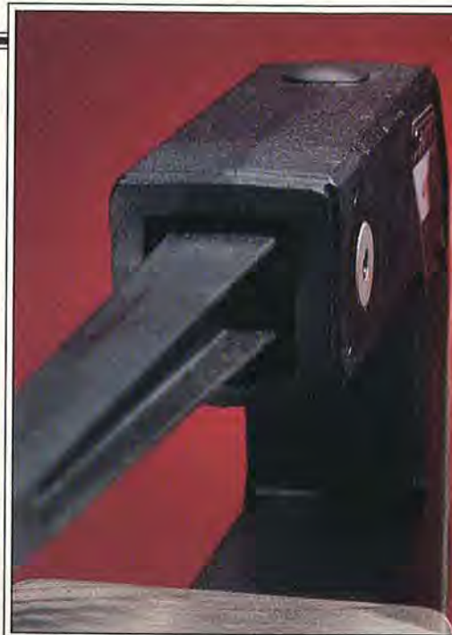
▲ The sleeve bearing holding the arm to the casting of the AMT model 4600 on the left supports the arm on both sides as shown.
