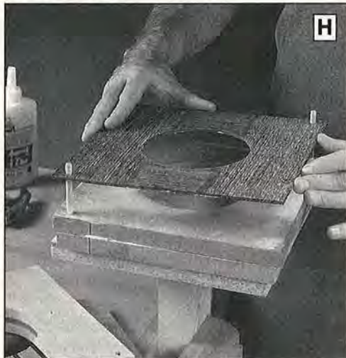
We used waxed 1/4" dowels as guidepins and lowered the successive layers on them as we glued. We sanded the ends of the dowels to round them off.
