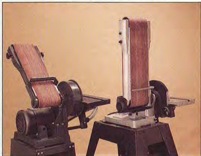
▼ The Lobo model SD-0069 on the left appears similar to the Jet model JSG-96 on the right, but the Lobo lacks a dust collection port and has a lightweight aluminum work table.
