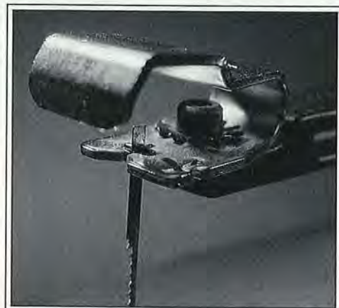
▲ The AMT model 4600 shown above has a pin-type blade holder, but you can install a pivoting blade clamping device that holds standard blades and comes with every unit.
