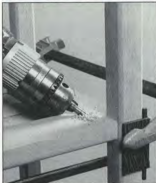
Angle the drill and drill a counterbored hole through the shelf and into the plant stand leg.
