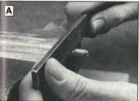
A Secure the all-thread rod in a vise or handscrew clamp, and file a \frac{1}{4} " notch \frac{1}{8} " deep \frac{1}{2} " from the end.
