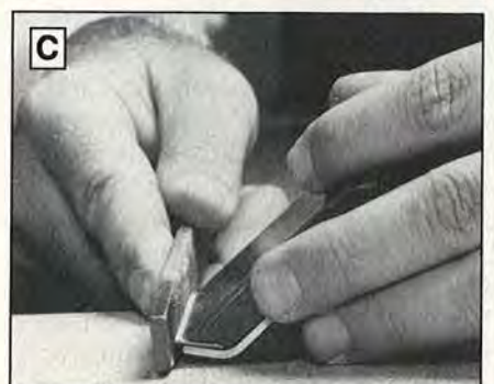
C Angle the scraper slightly less than 45^\circ . Using straight strokes, file the blade with a mill bastard file.
