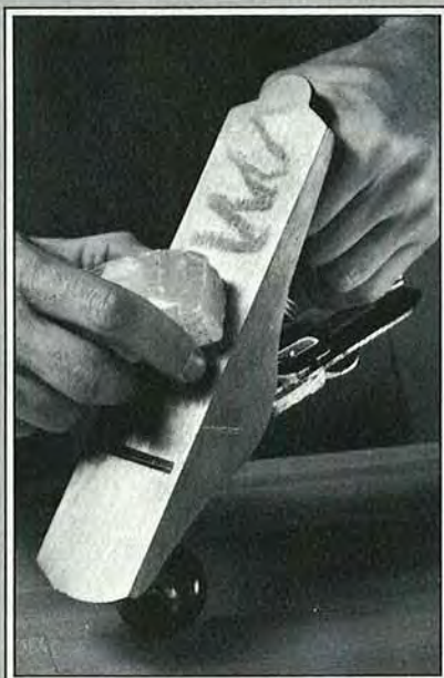
Apply paraffin to the sole of the plane to reduce surface drag.
