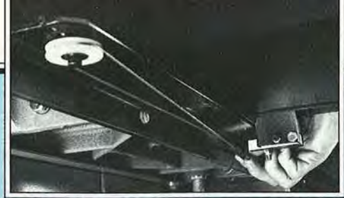
The Paralok fence quickly releases from its cable system with a tug on its cable connectors.
