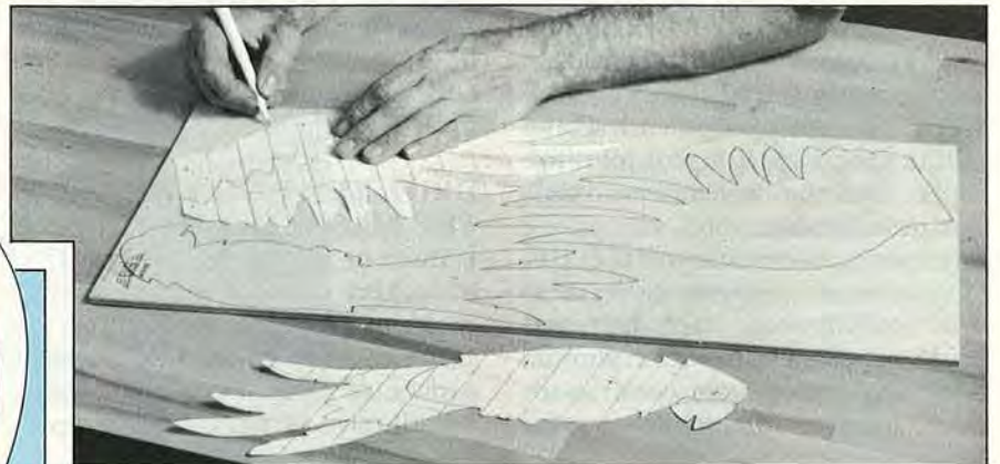
Using the templates, trace the outlines onto the plywood.
