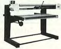
STROKE BELT SANDER SK-1500BS.....$1095.00 60"x21-1/4" sliding table 6" sanding belt width 2 HP SK-2100BS.....$1599.00 80" x 21-1/4 sliding table 6" sanding belt width 3 HP
