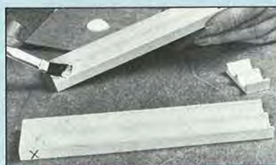
Apply glue to the mating surfaces. Then, glue and clamp the pieces with the edges and end flush.
