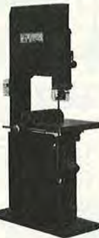
BAND SAW SK-20BS...$1195.00 20" cutting width 2 HP motor cast aluminum wheel
