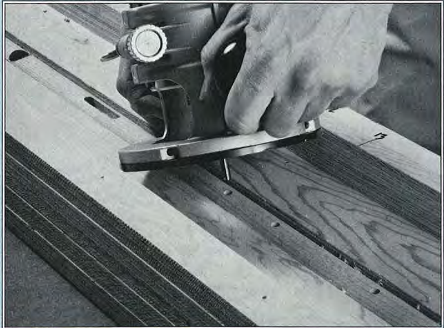
Lower the \frac{5}{16} " straight bit into the \frac{1}{4} " hole, and rout between a pair of \frac{1}{4} " holes to form the \frac{5}{16} "-wide mortises for the backrest slats.
