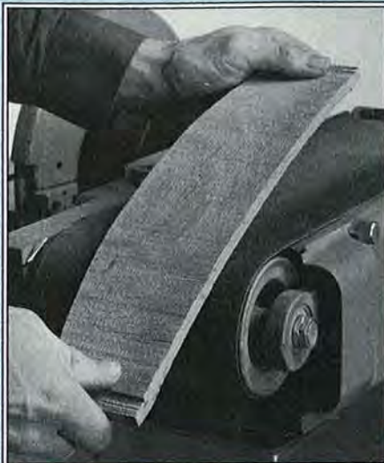
Sand the front and back surfaces of the backrest slats on a stationary or belt sander to remove the saw marks.
