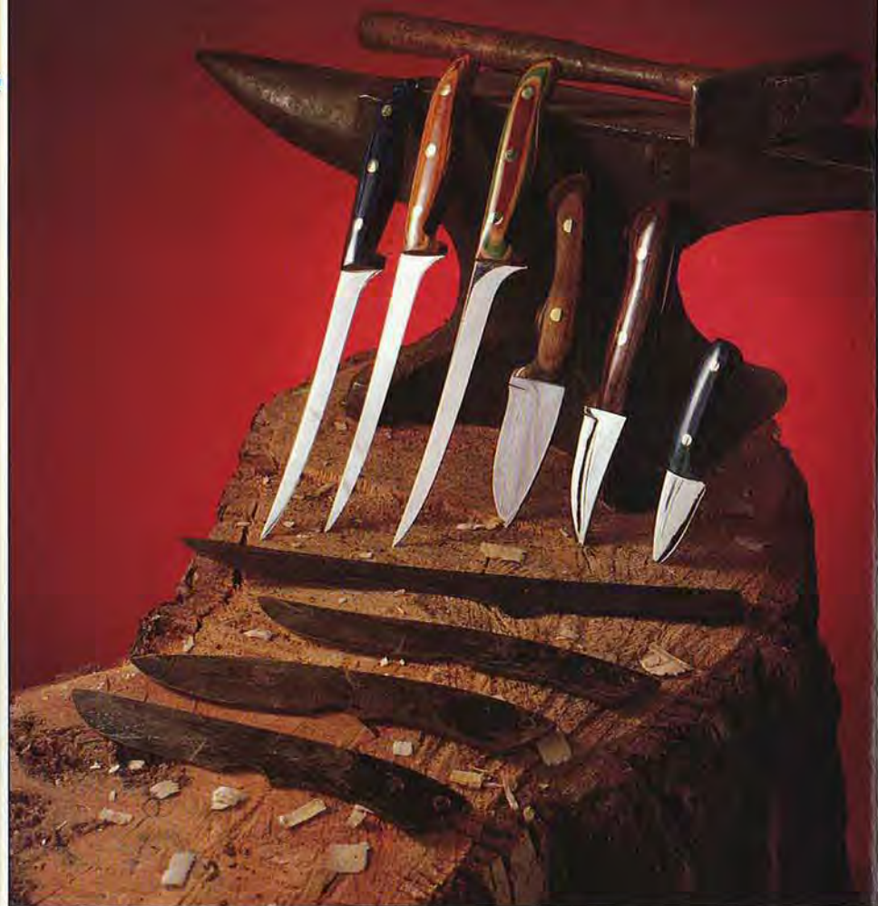
In the foreground, stamped, tempered blades ground to rough profile. Standing in back, fillet and hunting knives from Walt's product line.
