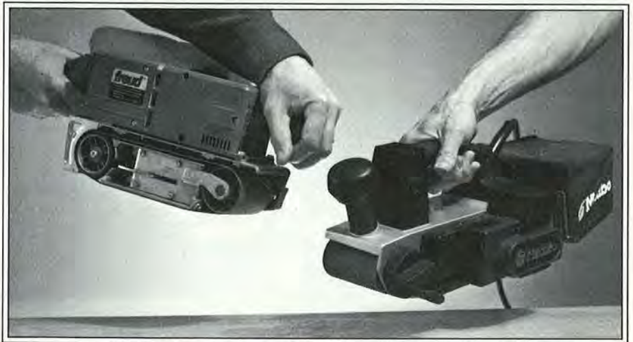
You'll need two hands to control inline sanders such as the Freud LC75 ( left ),
