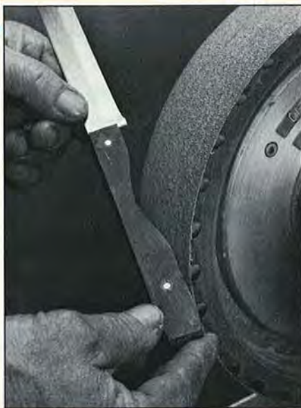
With a 60-grit belt, Walt grinds the laminated wood handle of a large meat slicing knife.
