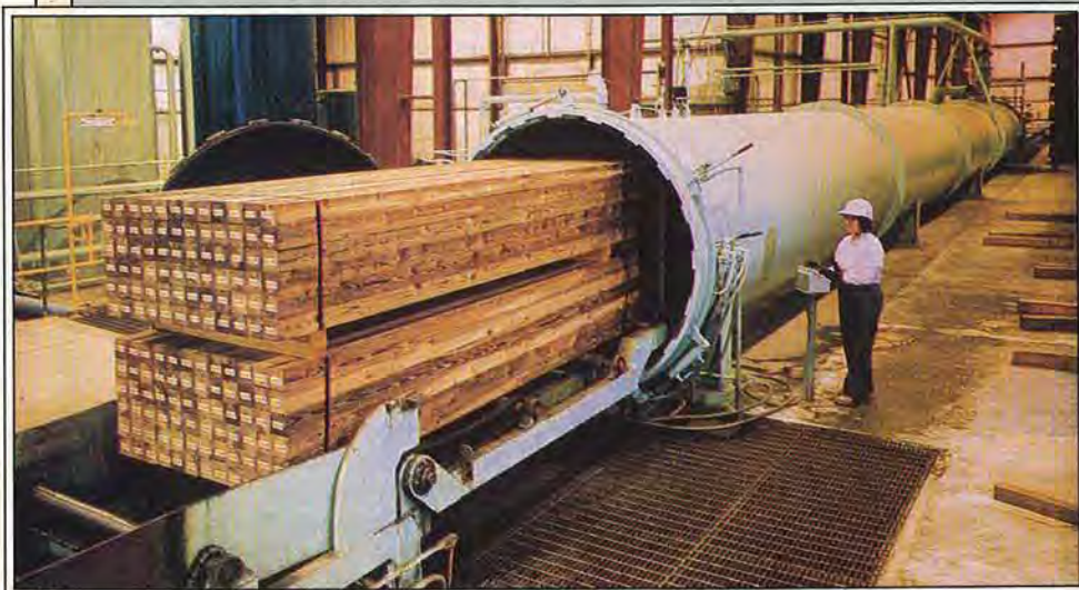
At Doyle Lumber Company in Henderson, North Carolina, 4×4 posts treated with Osmose chemicals leave a state-of-the-art indoor treatment facility.
