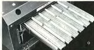
Woodmaster's Quick-Change Molding Head lets you create custom moldings from any stock. Choose from over 250 standard trim and picture frame patterns . . . or design your own!
