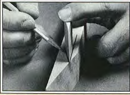
Mark the reference line, position the wedge along the line, and trace the wedge outline onto the side of the body.
