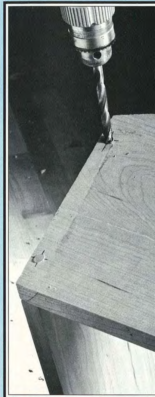
Carefully mark the dowel hole centerpoints on each side panel. Then, using a
