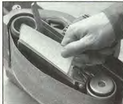
A thin piece of laminate between the platen and cork pad provided the final cure for this sander.
