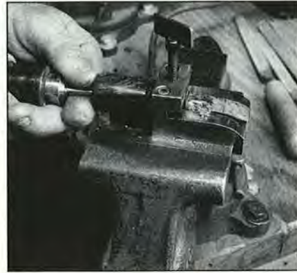
3. To allow air to flow against the reed, Butch drills a hole in the throat of the endpiece with a portable electric drill and a 1/4" brad-point bit.
