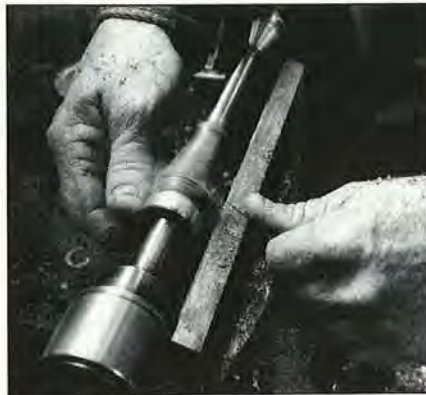
2. After scoring the barrel with a parting tool, the turner darkens the decorative lines by scorching them with a fine wire held tightly to the wood.
