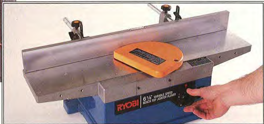
▲ Only one jointer—the Ryobi JP-155—has a variable-speed control: a plus as far as we're concerned.
