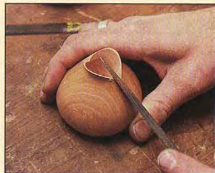
Mark employs half-round files to smooth the belt-sanded edges of each candle holder.
