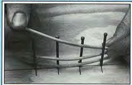
Soak 1/2" dowel stock in water, and then bend the dowels around the nails to shape the headlight bars.
