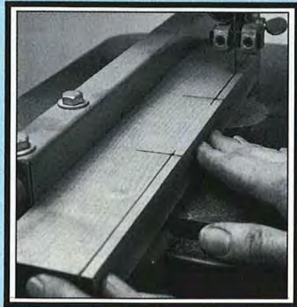
Position the fence and align the blade with the center of the \frac{1}{8} " holes. Bandsaw to the holes to form a pair of kerfs in the alignment block.
