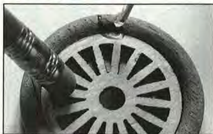
Dab instant glue onto the joint between the tire and the laser-cut insert.
