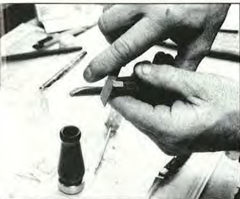
4. Butch's work-worn hands perform the delicate work of tuning a call. For proper sound, the cork, shaved to fit, must hold the Mylar reed exactly right.
