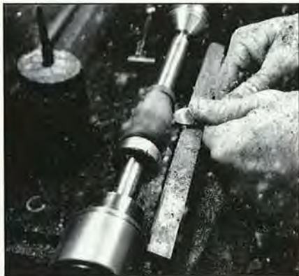
1. With a turning tool made from a used commercial planer blade, Butch shapes a call barrel. To make his calls, Butch relies on three Rockwell lathes.
