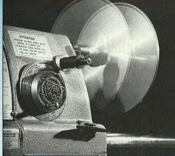
The quill-mounted disc sander moves to the workpiece, giving you greater control over certain sanding operations.
