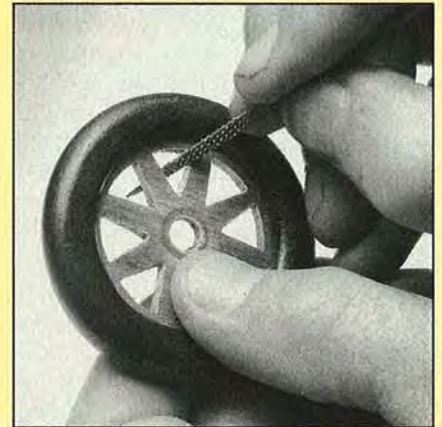
Small riffler files help you clean up scrollsaw cuts, even in the tightest spots between the wheel spokes.
