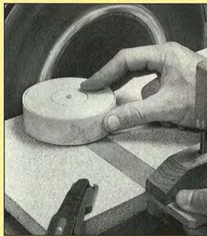
Set the sanding jig's stop for the correct wheel diameter, then turn the wheel into roundness with a disc sander.
