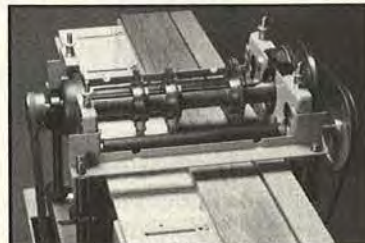
GANG RIP SAW — Edge cut and dimension the width of your stock!
