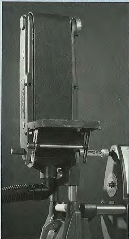
Although nearly identical to the Total Shop belt sander, the Shopsmith unit has a swiveling 2½" dust port.
