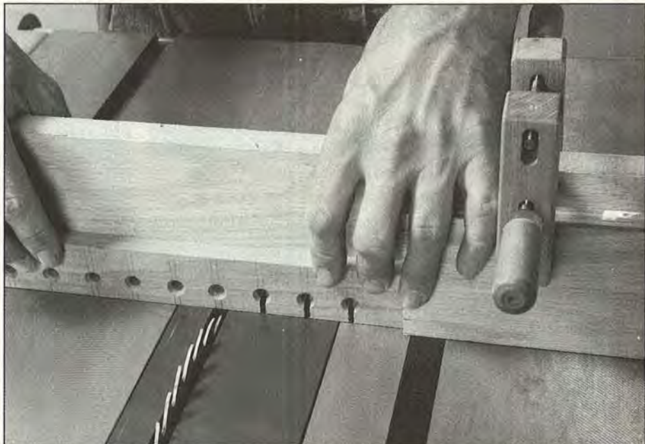
Mount an auxiliary fence to your miter gauge, and cut the kerfs.
