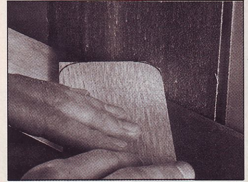
Use a disc or vertical-belt sander to shape flowing convex curves.
