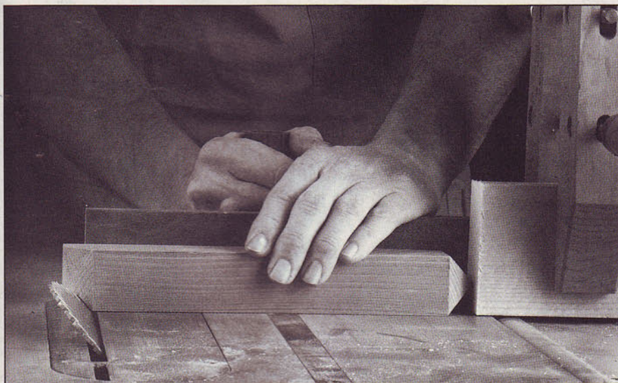
Angle-cut the ends of a 12" length of 1½" square stock to form the pointed ends on each part H. For safety, we started with an extra-long piece.
