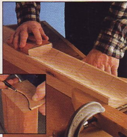
As you sand the cove molding, be careful to remove only the saw marks. Smooth with 100- and 150-grit papers.
