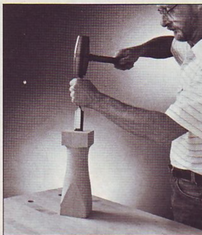
Using a mallet and 1" chisel, split the lamination at the four paper joints.
