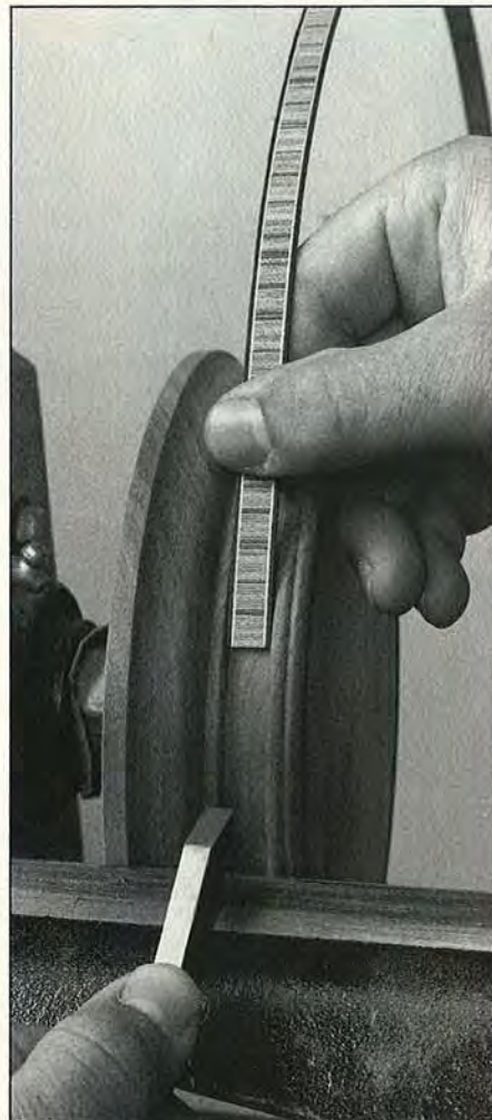
Stop the lathe frequently when turning the inlay-border groove with the parting tool to check the fit of the inlay.
