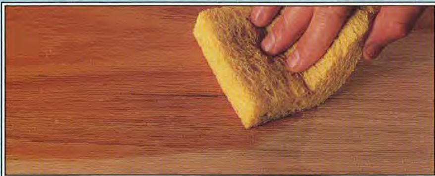
Apply a thin film of water with a sponge or rag to raise the grain.
