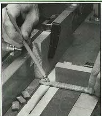
To safely cut the short spacers, use the eraser end of a pencil to clear the spacers from the blade.
