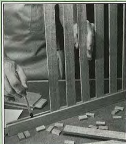
Brush epoxy into the groove in the backrest lower rail, and then add the spacers and splats.
