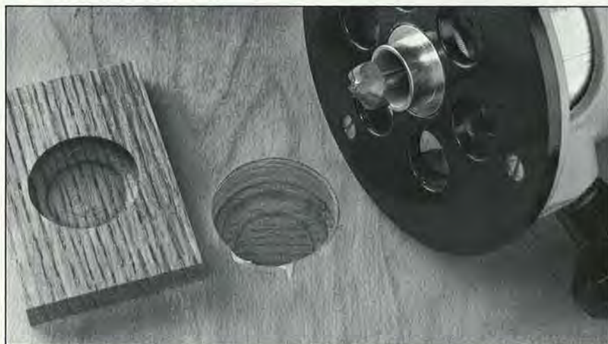
Position a drawer front into the routing jig and rout the depression. A routed front and the router are shown at left.
