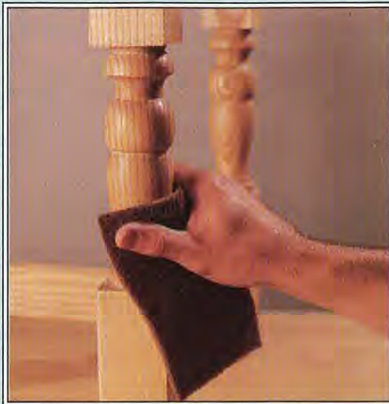
On contoured surfaces, smooth the finish with 3M Scotchbrite pads instead of steel wool.
