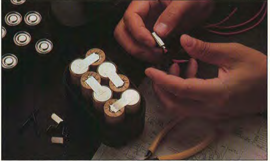
During battery-pack assembly, a worker adds a small thermostat that tells a charger when to stop charging, preventing any damage to the battery cells.
