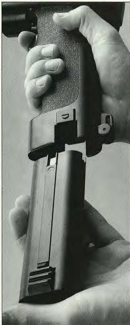
The battery pack on the Sears model 11128 had a tendency to fall out of the handle when the tool was jarred.
