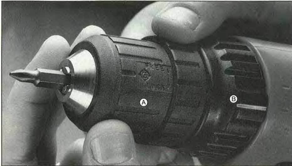
The keyless chuck (A) of the Hitachi D 10DF worked smoothly and effortlessly. The clutch control (B) helped make driving screws a breeze.
