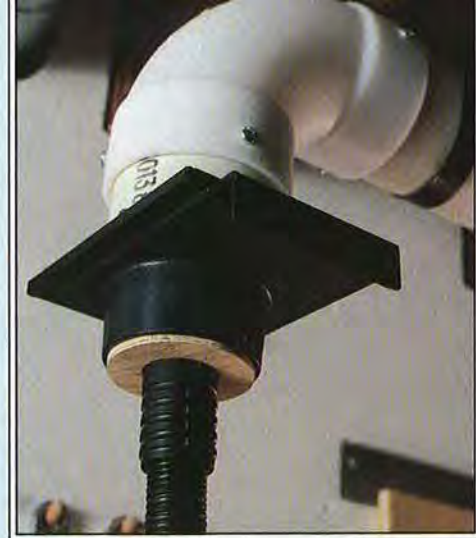
A 3" blast gate outfitted with a wooden doughnut accepts a 1" hose for portable tools such as sanders.
