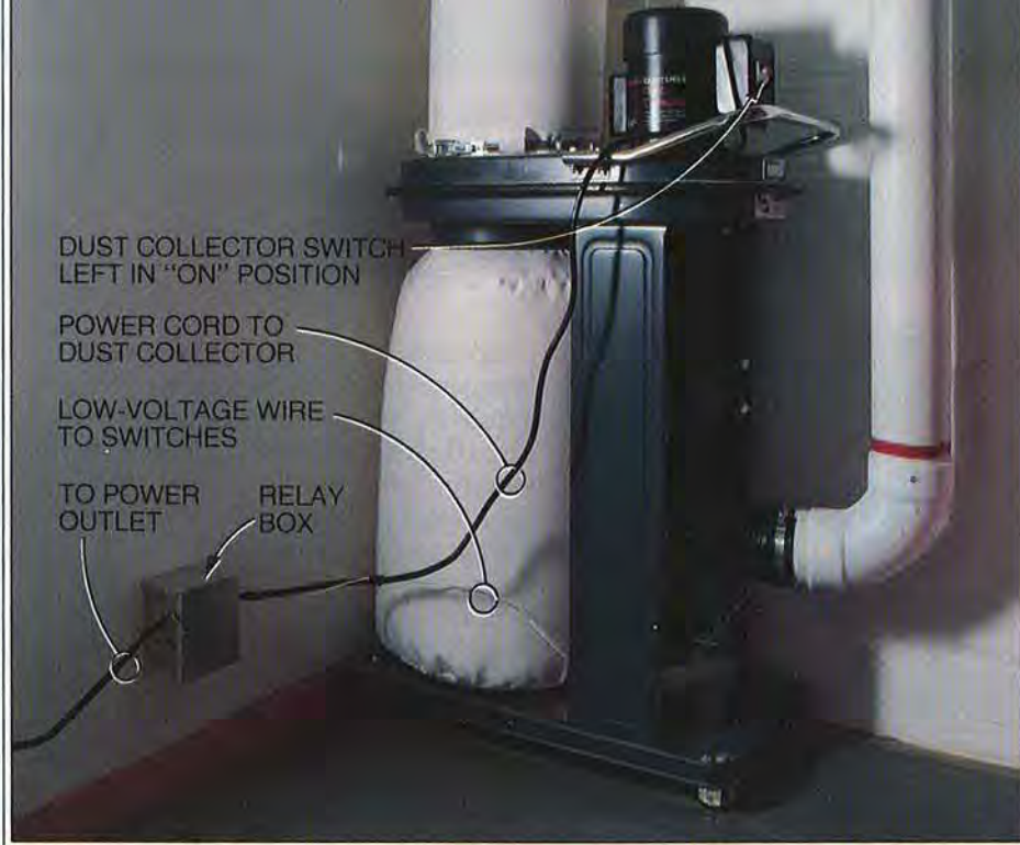
If you decide to install multiple switches, mount the relay box for the low-voltage switching system on a wall near your dust collector.
