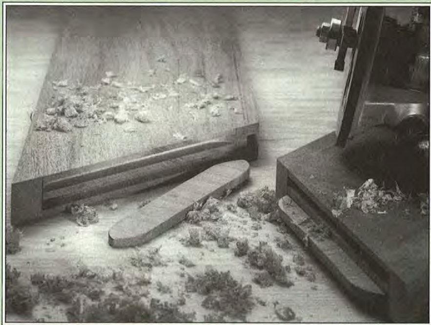
Rout a pair of slots and cut a pair of splines for each mitered corner joint.
