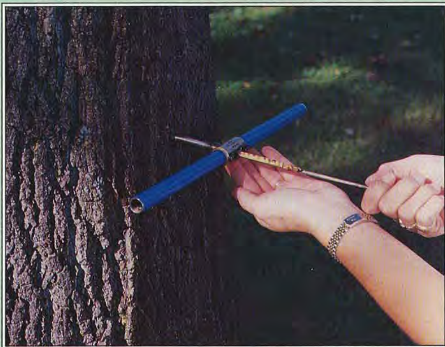
To obtain rings for reading, a researcher bores into the center of a tree with a hollow \frac{1}{4} " auger bit.
