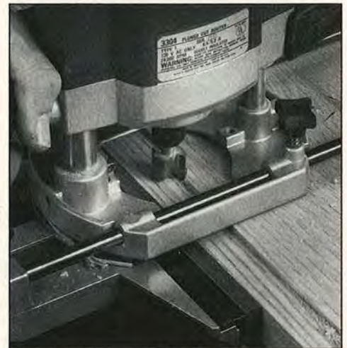
Fit your router with an edge guide and a straight bit. In several passes, rout a \frac{1}{8} " rabbet 1" wide along the tabletop edges.
