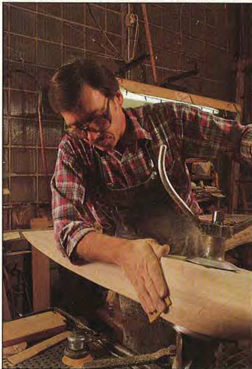
Al Dissinger gives a propeller an extensive sanding with 100-grit paper before it goes to the finishing room.
