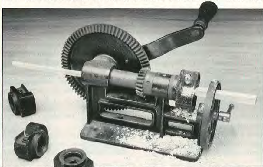
Some craftsmen still use the Stanley No. 77 dowel and rod turning machine, pictured here with three extra cutter heads.
