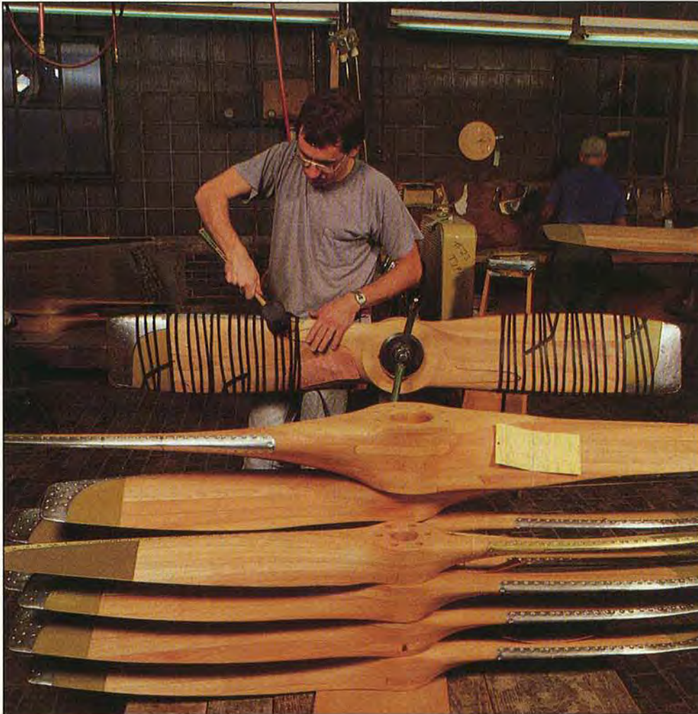
Airboat propellers receive metal tips and protective edges. Here, Randy Goshert checks the tightness of the wrapping that holds the metal edge so that it can be riveted and screwed in place.
