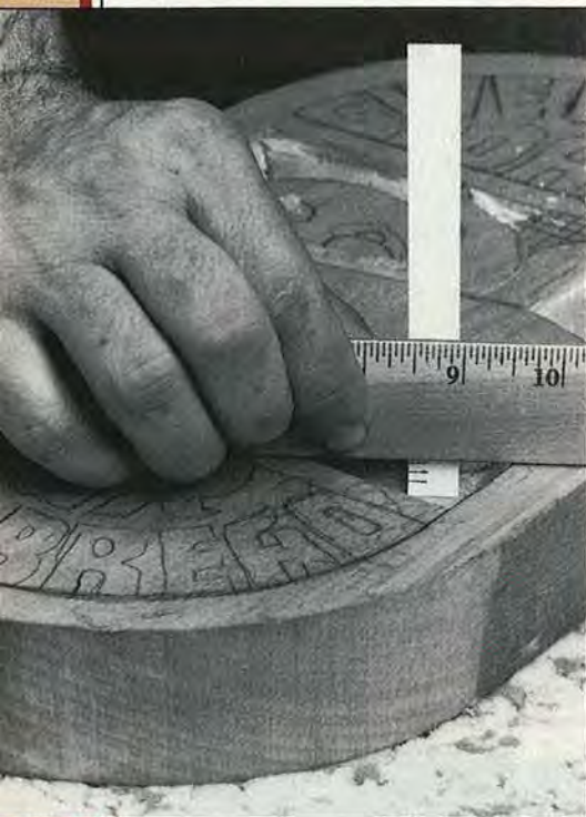
▲ Check relief levels during grounding with the depth gauge and a straightedge. The color-coded pattern shows depths for grounding the plaque.
