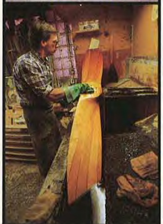
A Sensenich propeller has 5 to 13 laminations and two protective coats of dipped-on spar varnish.
