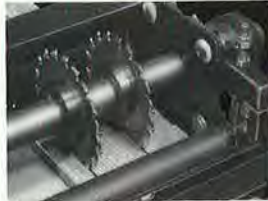
New rip saw attachment lets you gang-rip with power feed in a fraction of the time it takes for multiple hand-fed passes on an ordinary table saw.
