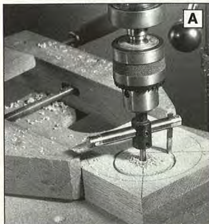
Use a circle cutter to form the 2\frac{7}{8} " hole in the laminated base block.
