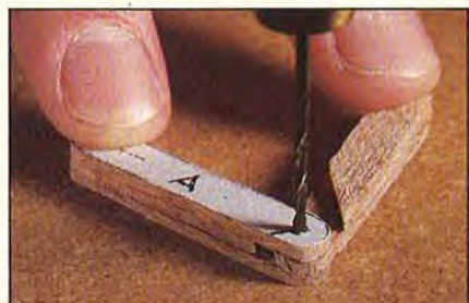
Align the rounded ends of the hinge to drill the hole for the brass pin.
