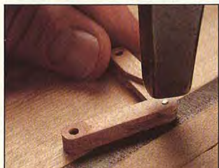
Peen the ends of the pin to prevent it from falling out of the hinge.
