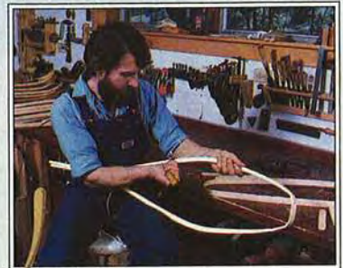
Snowshoes require much handwork. At his workbench, Carl rounds the frame edges with thin slices from his shop-made crooked knife. The contour inside the frame was done with a draw-knife at the shaving horse.
