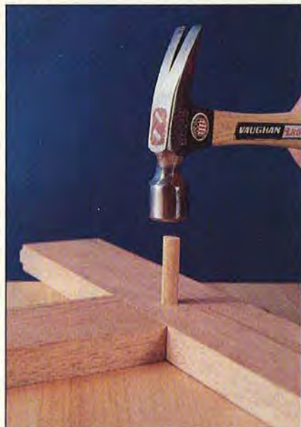
After applying glue to the dowel, tap it into place, saw it, and sand flush.
