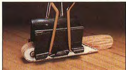
Binder paper clips (as shown) and clothespins make good, inexpensive clamps for all your small projects.
