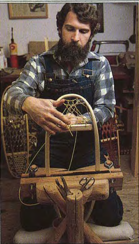
Lacing takes half the total time involved in snowshoe making. Carl makes the task easier by inserting frames in the vise on the lacing frame, where he can kneel as he pulls the wire taut.
