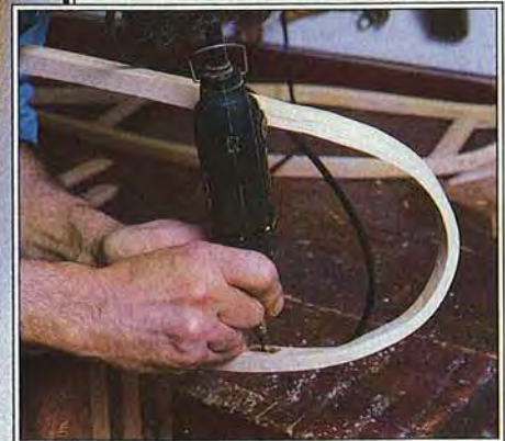
About the only power tool Carl uses extensively is a Dremel Motoool. With it, he cuts the mortises for the crossbraces, and recesses for the laces.
