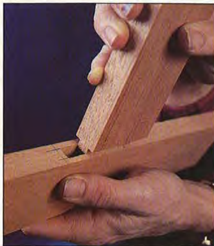
Check the width of your mini tenon before cutting the full tenon.
