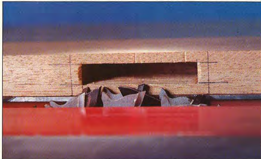
Lay your mortised workpiece on the top of your tablesaw and adjust the height of the dado blade or set according to the setback of the mortise.
