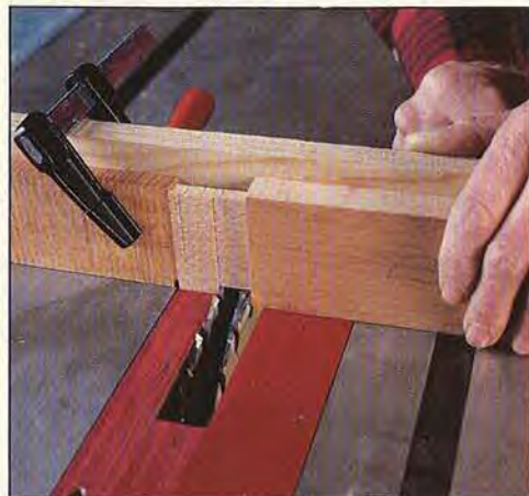
After clamping a stopblock in place, cut all four shoulders.
