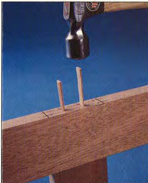
After cutting narrow wedges with your bandsaw, gently tap them into place.
