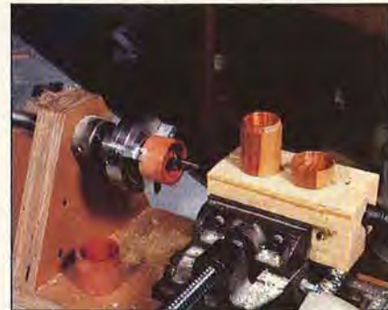
The power source for Bonnie's threading jig is a flexible-shaft carving tool in a wooden mount.
