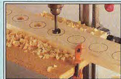
Mark the wheel centerpoints and radii, and use a 1" Forstner bit to drill holes \frac{1}{2} " deep for each wheel.
