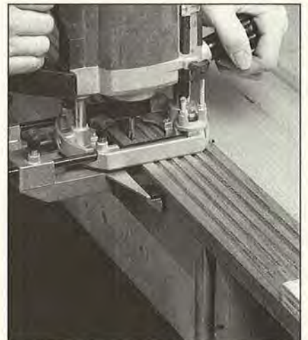
Rout \frac{1}{4} " veins \frac{3}{16} " deep using a router fitted with an edge guide and stops clamped to the ends of the stile.
