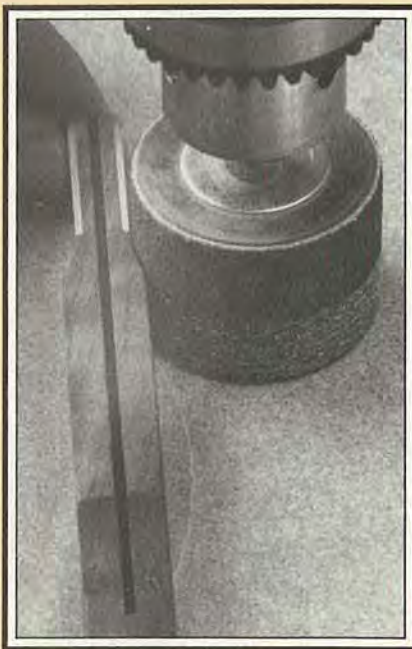
Mark the radii on the walnut portion of the handle, and then sand to the line being careful not to sand the brass.
