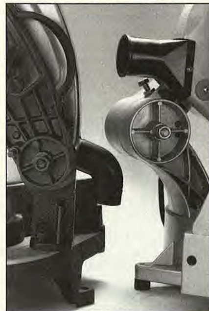
The Hitachi C10FA angle-only miter saw, right , has a heavier knuckle assembly than the Ryobi TS254, left .
