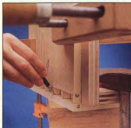
Clamp the workpieces to the bracket for accurate tail marking.
