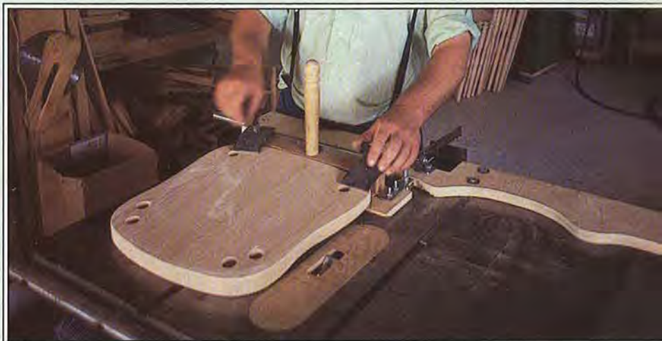
► David built a jig for the seat blank to follow in back-and-forth travel as the solid dado head in his tablesaw contours the glued-up blank of wood.
