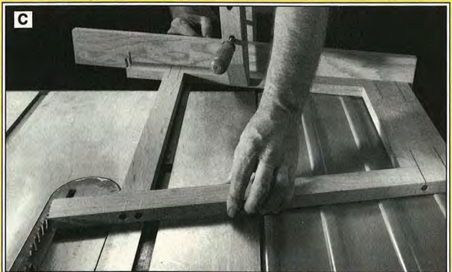
Adjust the miter gauge 10° right of center, and bevel-rip the bottom edge of the leg assembly parallel to the top edge.
