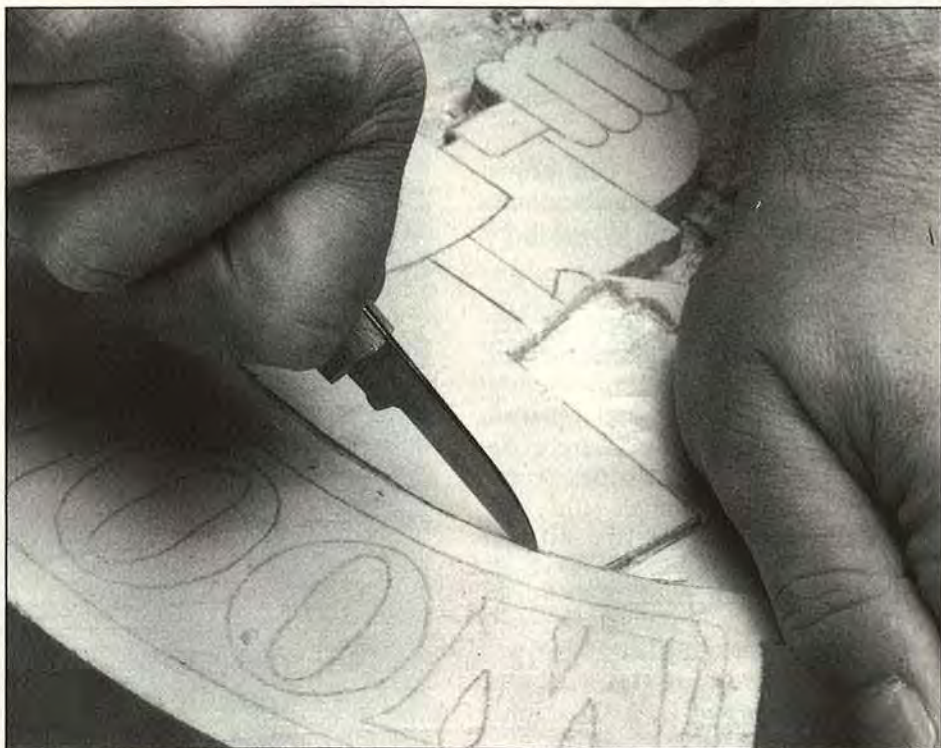
▲ Create straight sides for your relief areas by stop-cutting along pattern lines. Be careful not to slope or undercut the sides.
