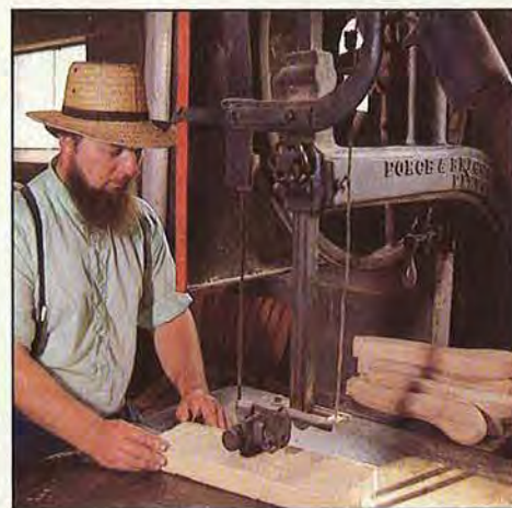
▲ David's old bandsaw long ago shed its electric motor. It now runs on economical pneumatic power, as do most of his machines. Others run on hydraulics.
