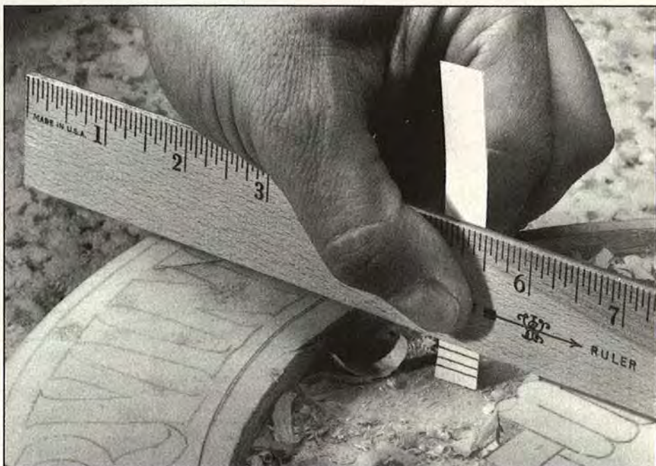
▲ Check carving levels with the depth gauge, which is keyed to the color-coded pattern. Measure each level at several points.
