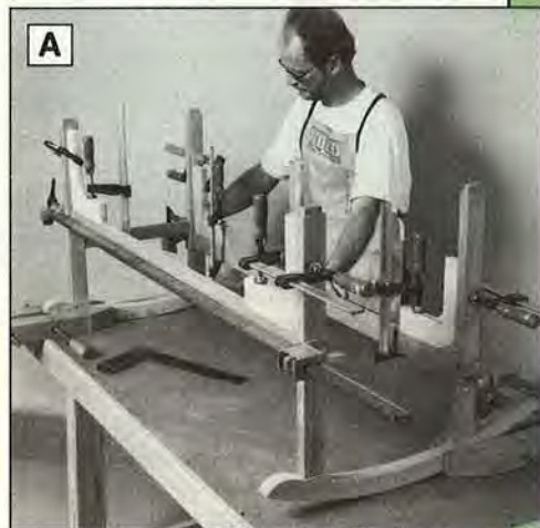
We used 90° corner braces to hold the rocker frame pieces square while the glue dried.
