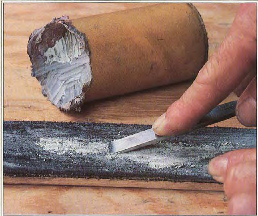
As you strop the tool, mash the bits of compound into the leather surface. Press hard as you pull the tool along the strop five or six times.
