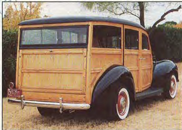
► A restoration by Mark Miller of Penrose, Colorado, this 1939 Ford has maple framing and one-piece, figured birch plywood panels. Ford switched to mahogany panels in 1942.
