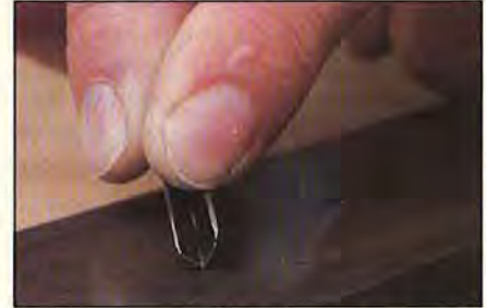
Gently round the outside of the V on a fine India stone, so it matches the roundness on the inside of the V.
