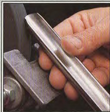
Keep the tool moving as you grind it to avoid overheating.
