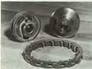
"We reduced the vibration in our table saw by replacing its cast iron pulleys (left) with turned pulleys (right) and adding a link belt."
